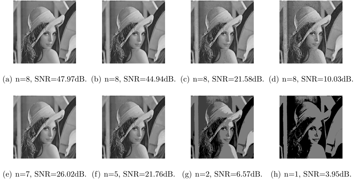
Figure 3.18: Output images of the FIR filter for both overclocking scenario (top row) and traditional scenario (bottom row) when operating frequencies are 425MHz, 450MHz, 480MHz and 520MHz, respectively (from left to right).
