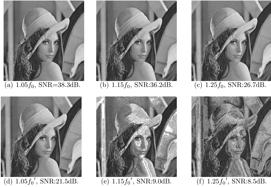
Figure 4.6: Output images of image filter using online arithmetic (top row) and traditional arithmetic (bottom row).
