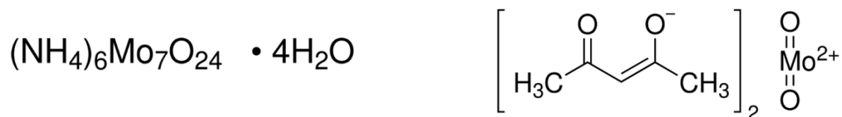
Figure 20: Ammonium Molybdate Tetrahydrate (Left) and Bis(acetylacetonato)dioxomolybdenum(VI) (Right), the two precursors investigated for deposition of MoO 3 by spray pyrolysis.
