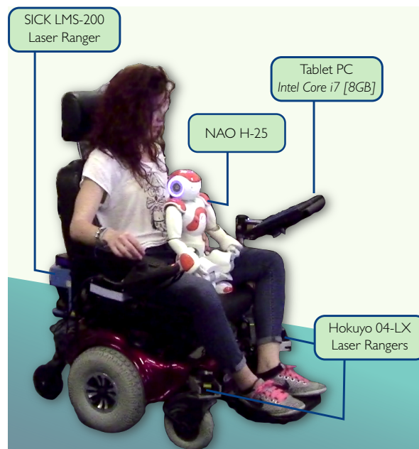
Figure 5.3: Hardware components of our robotic tutoring system.
