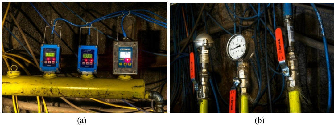
Figure 8.5: The gas drainage real-time monitoring equipment: (a) Gas concentration sensors (from left to right: CO 2 (0~100 %), CH 4 (0~100 %), and CO (0~200 ppm)); (b) Gas pressure and temperature monitoring (from left to right: pressure sensor (-1~1 bar), pressure gauge (-1~5 bar), and temperature sensor (0~100°C)) (Courtesy of Coal Mine Velenje Researchers).
