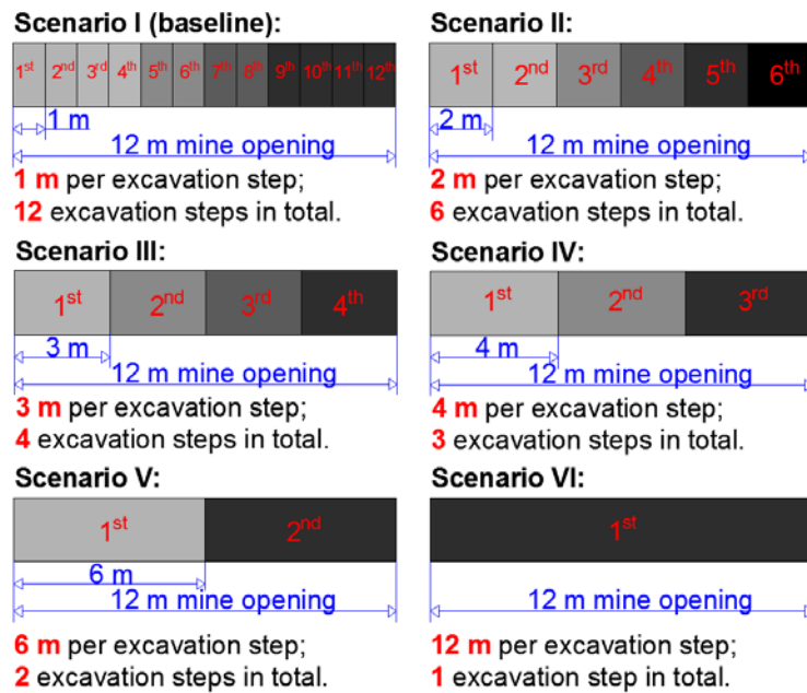
Figure 6.7: Illustration of different coal extraction strategies used in the numerical experiments.
