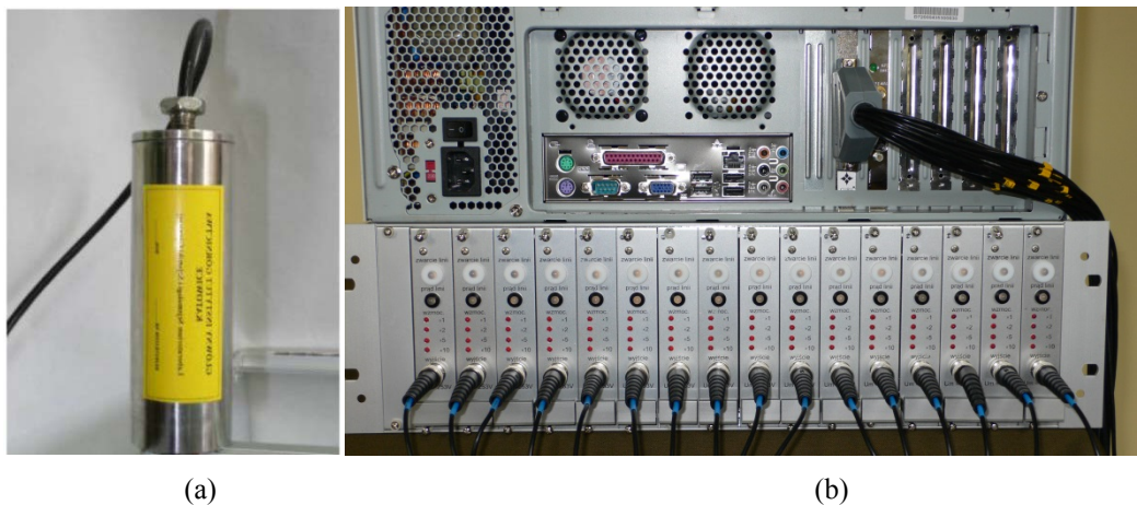
Figure 5.8: Microseismic monitoring equipment: (a) the low frequency DLM-2001 geophone probe and (b) DLM-SO surface data receiver (after Si et al. , 2015b).
