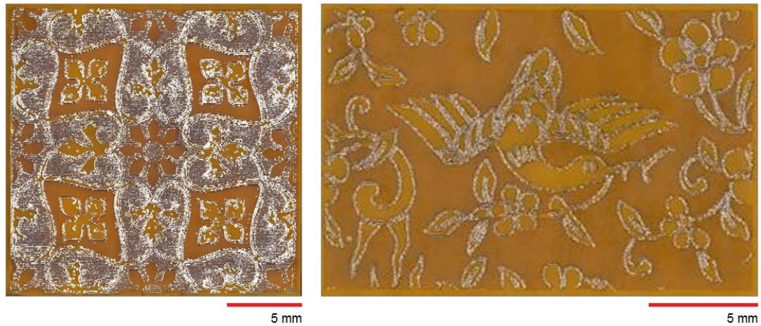
Fig. 45. (a) and (b) Two samples of glass embedded with silver nanoparticles which have been irradiated for the purpose of visual effect. The different 'shades' are produced by varying the laser energy fluence which creates these aesthetically pleasing designs.
