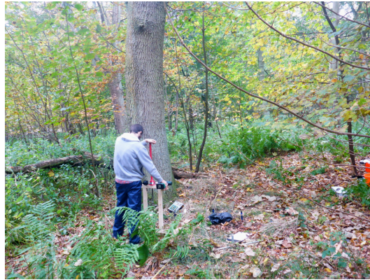
Figure 7.2: Blade penetrometer testing near oak tree at Paddockmuir Wood.
