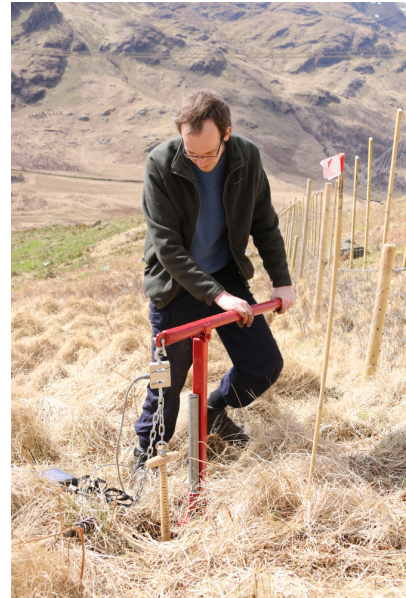
Figure 8.40: Picture of corkscrew testing on 'natural' slope at QEFP.
