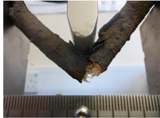
Figure 7.9: Three-point bending test on oak root.
