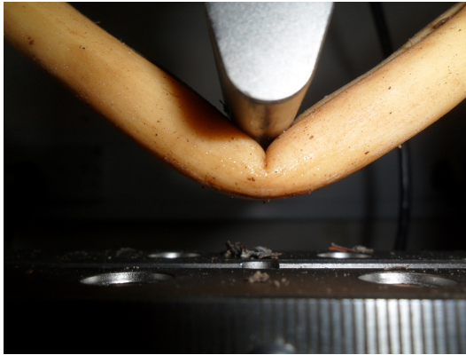
Figure 7.8: Three-point bending test on barkless Sitka spruce root.
