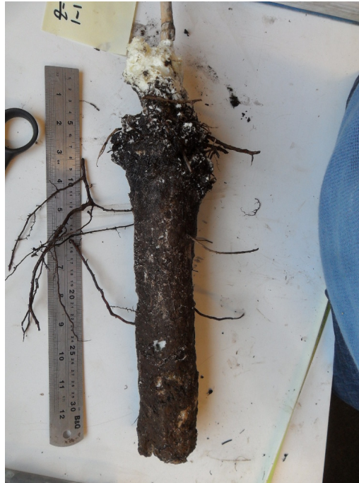
Figure 8.19: Example of a foam core after washing away surrounding soil, used to identify roots broken during corkscrew testing.
