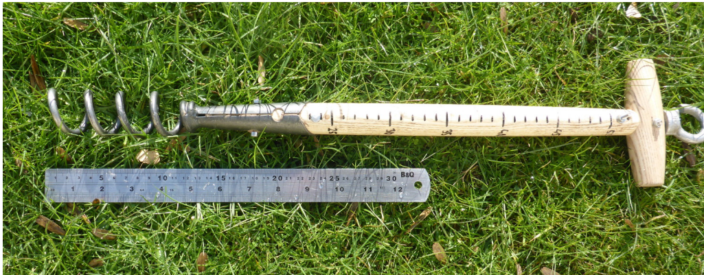
Figure 3.8: Picture of the corkscrew device used.
