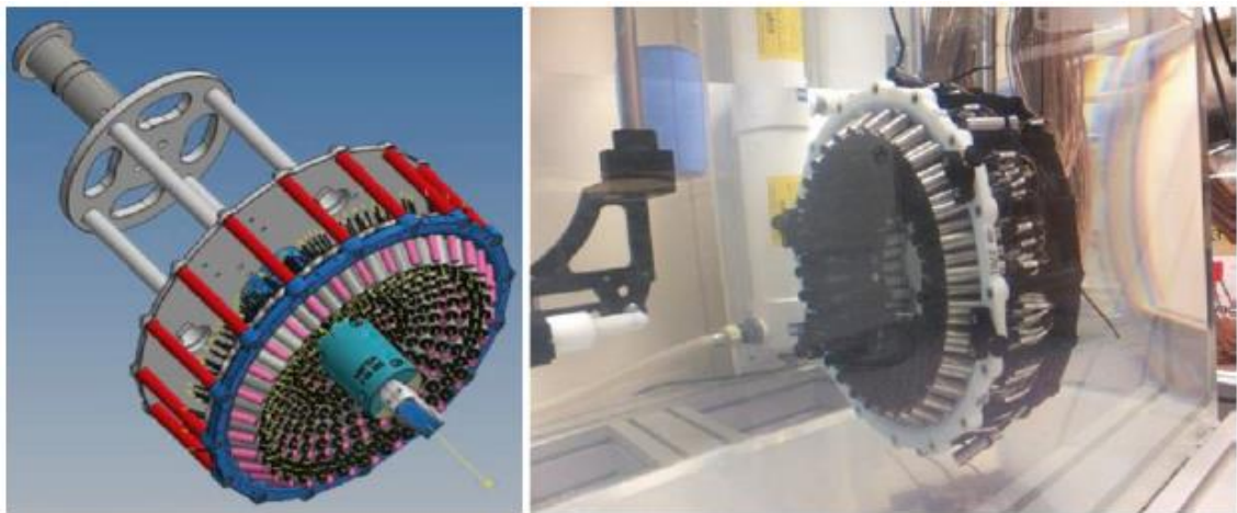
Figure 2.2. Multi element phased array. Consists of 256 individual elements, enclosed in a 3D printed shell. Taken from (Escoffre and Bouakaz, 2015).
