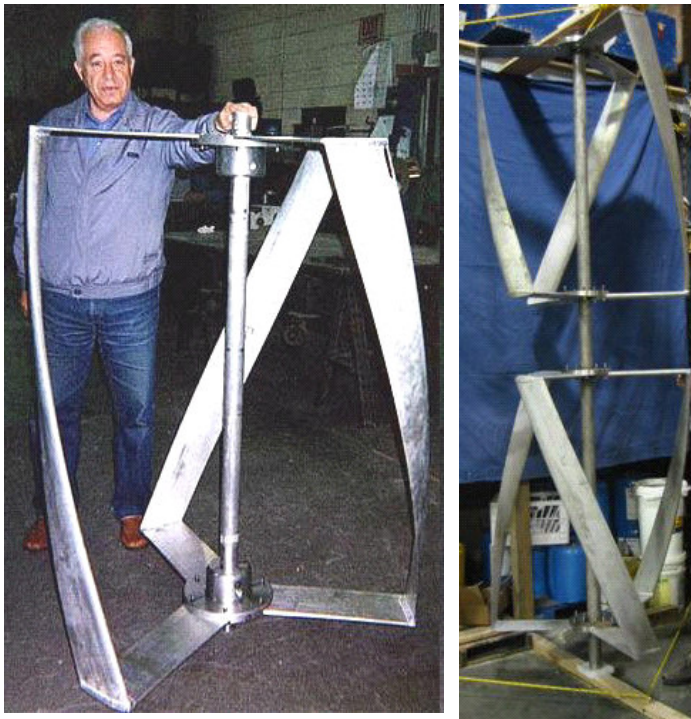
Figure 43: Gorlov Helical Turbine - Dr. Gorlov, left - Gorlov turbine double rotor, right
