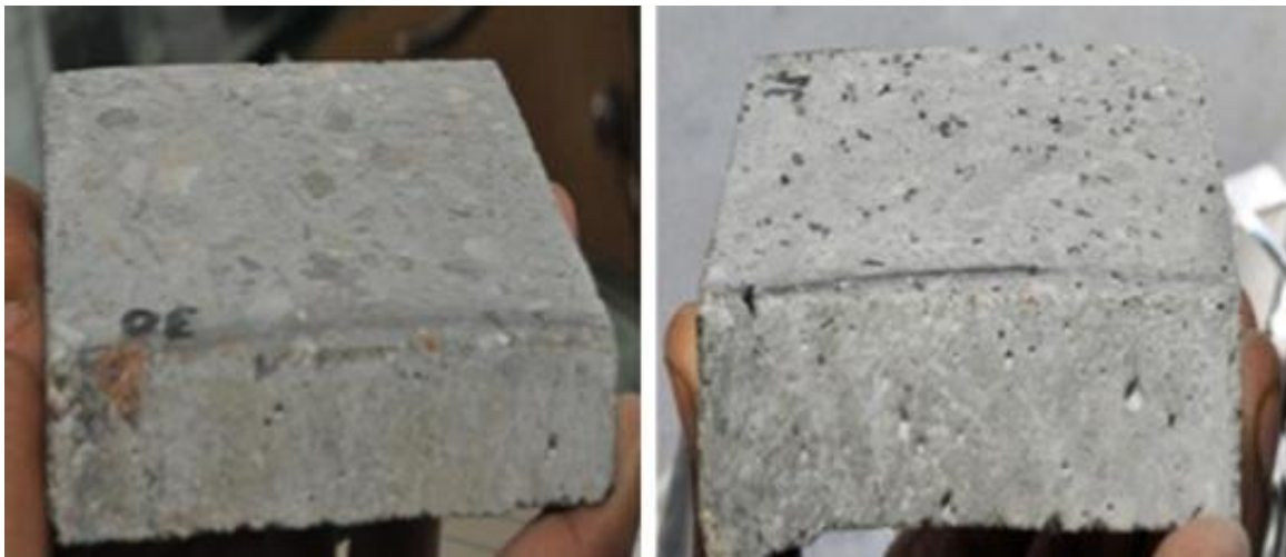
Fig. 4. Surface of the control mix (0% rubber) and rubberized concrete after Abrasion test [6]
