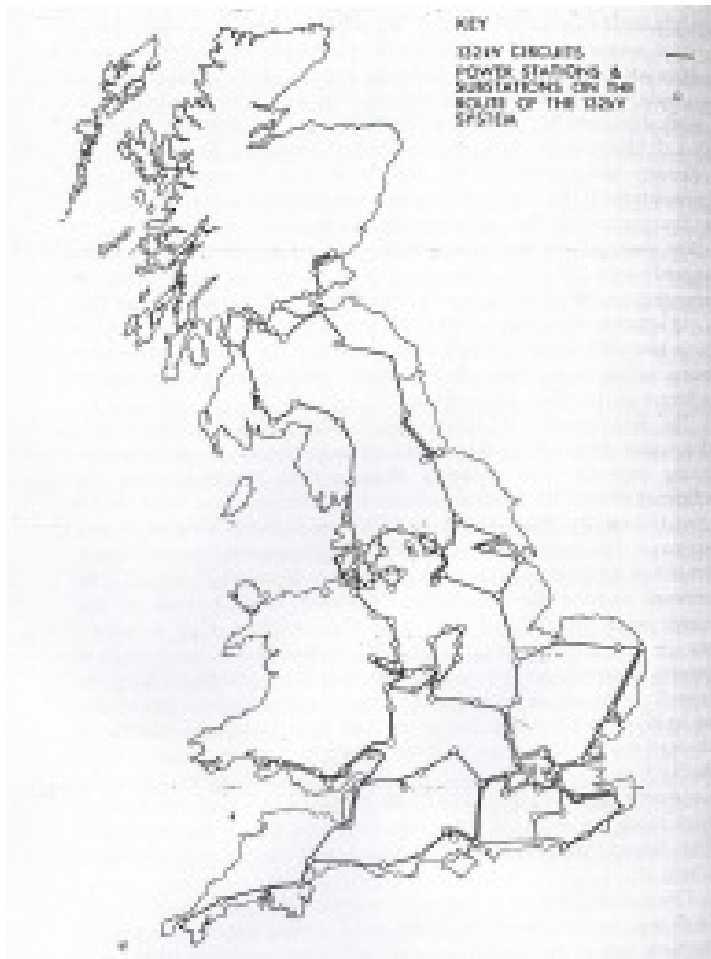
Figure 11: The 132kV grid at its inception, 1932. Source: Hannah (1979)
