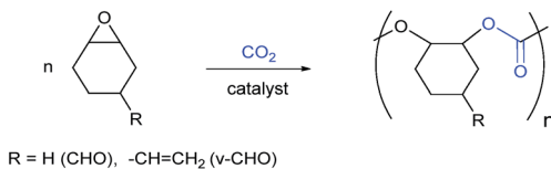
Scheme 1 Illustrates the ring opening copolymerizations using cyclohexene oxide (CHO) and vinyl-cyclohexene oxide (v-CHO).
