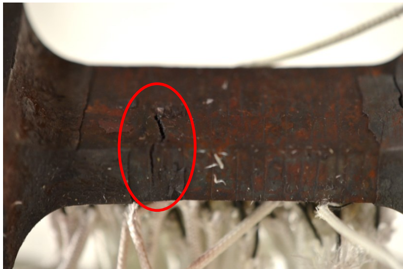
Figure 6.14: Photograph of specimen after experiment was concluded. A crack can clearly be seen in the vicinity of the HAZ.
