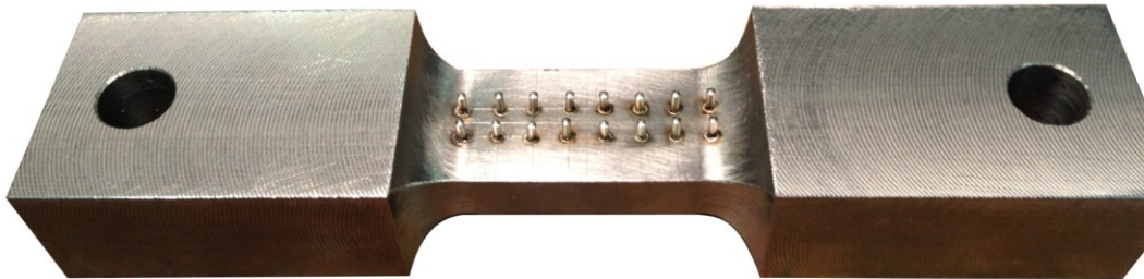
Figure 2.16: Photograph of a high temperature creep specimen with an array of 5 mm electrode separation potential drop sensors along one face.
