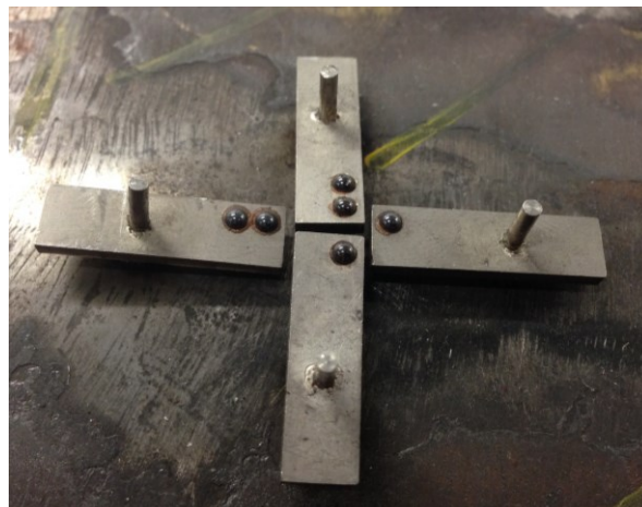
Figure 1.6: A photograph of a biaxial ARCMAC gauge. The two spherical SiNi targets on one carrier plate provide a strain independent reference measurement. The distance between targets on opposing carrier plates provides the strain measurement.
