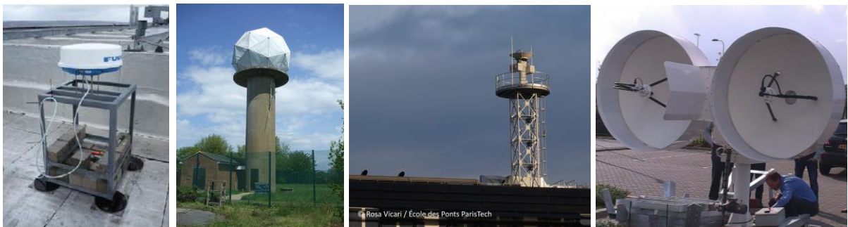
5 Figure 2. Radars implemented at the pilots sites of RainGain (from left to right): X-band 6 single pol radar implemented in Leuven, Chenies C-band radar of the UK national network, 7 dual-pol X-band radar installed in Paris, dual-pol X-band radar to be installed in Rotterdam.
