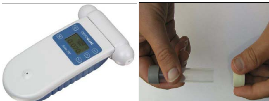
Figure 4.1 NO 2 monitors for the pilot study: Aeroqual Series 500 with NO 2 gas sensor (left) and Passam tube (right)
