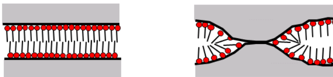
Figure 2 (a) Hardy and (b) Bowden and Tabor models of OFM mechanism
