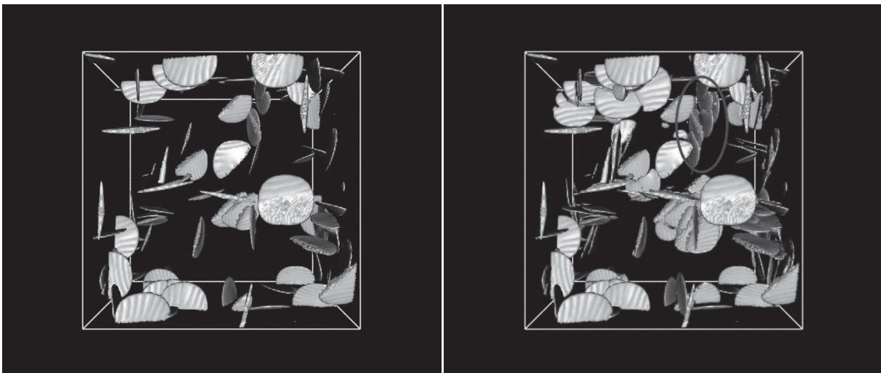
Fig. 3. Figures of bainite formation at 10,000 time steps (left) and 28,000 time steps (right) in two austenite grains. The part of the domain marked in red indicates the growth of two sheaves via autocatalysis.
