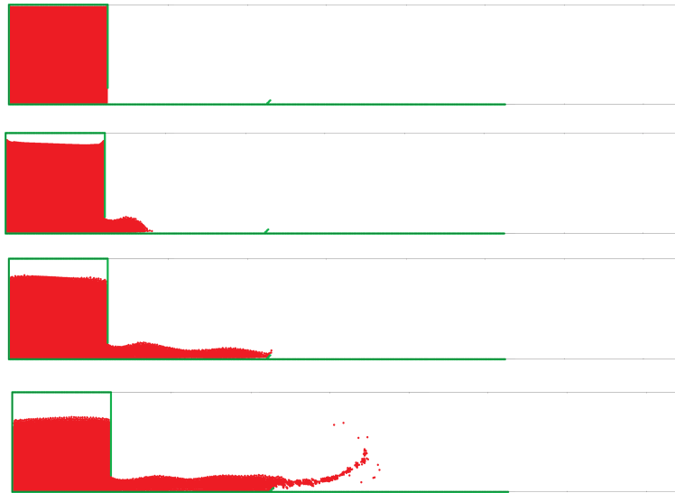
Figure 4.12: Dam raise simulation with 10000 particles at time steps 30 (top), 990 (second down), 2490 (third down) and 3990 (bottom). Virtual boundary particles (green) were used. Friction exists in the form of particle-boundary interaction.
