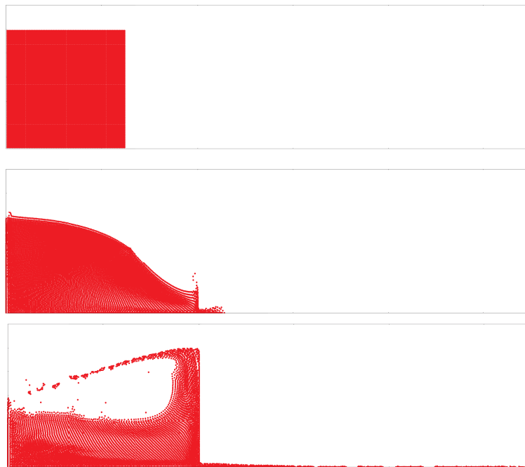
Figure 4.11: Dam collapse simulation with 10000 particles at time steps 30 (top), 1620 (middle) and 3990 (bottom). No boundary particles were used in this SPH simulation, instead a simple bounce back algorithm was applied at the boundaries (invisible). This corresponds to the absence of friction.
