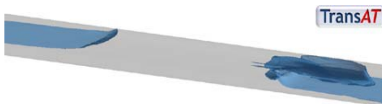
Figure 3.25: The formation of initial slug, liquid hold-up equal to unity.
