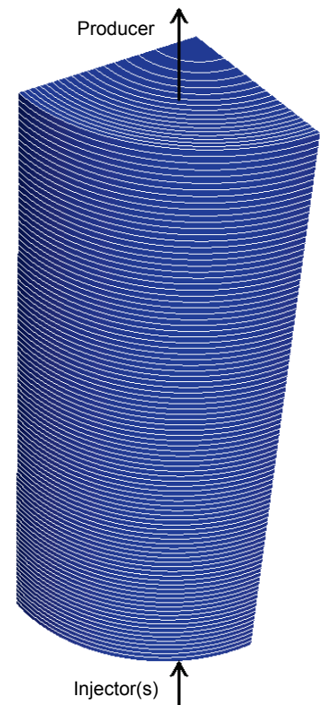
Fig. 2 —Illustration of the core model grid. Both water and CO 2 are injected from below.
