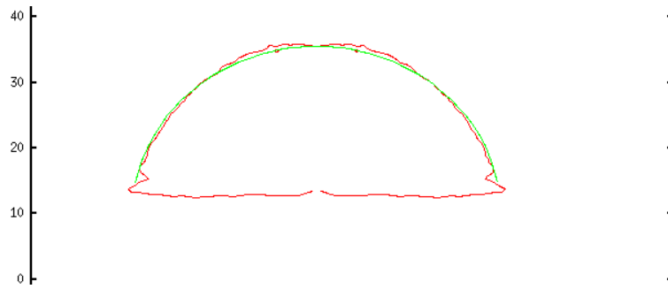
Figure E 7: Simulated image of water droplet under a CO 2 density of 880.52Kg/m 3 at 320K.
