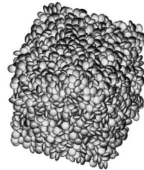
Figure 1 – Geometric random packing of 4000 oblate spheroids. (Stoyan 2006)
