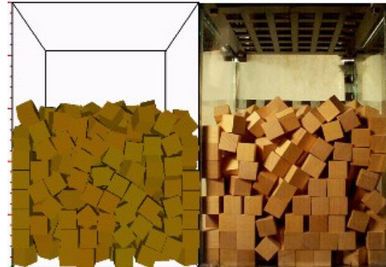
Figure 3 – Comparison of cube packing structures from Y3D simulation and experimental setup. (Latham and Munjiza 2004)
