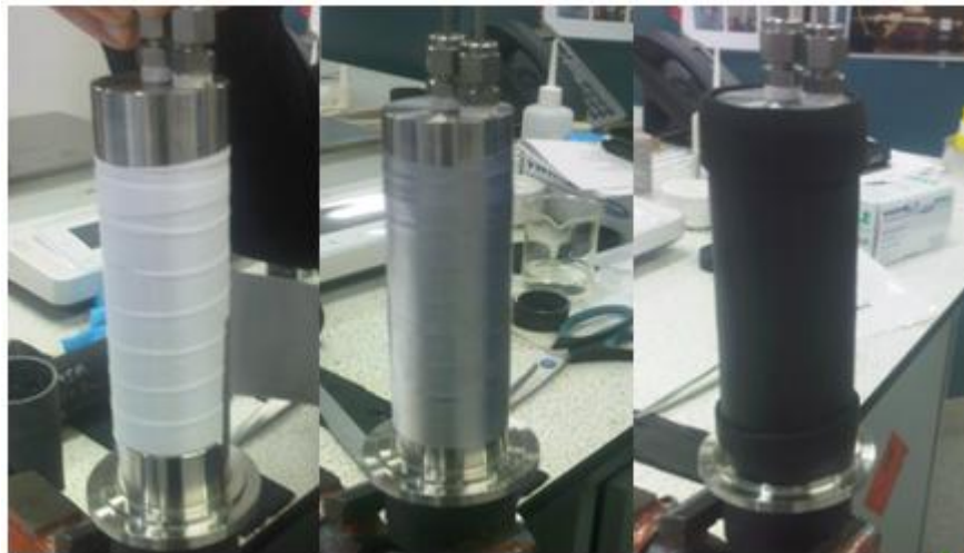
Figure AP- 1 shows the process of core preparation prior to placing it inside an oven.
