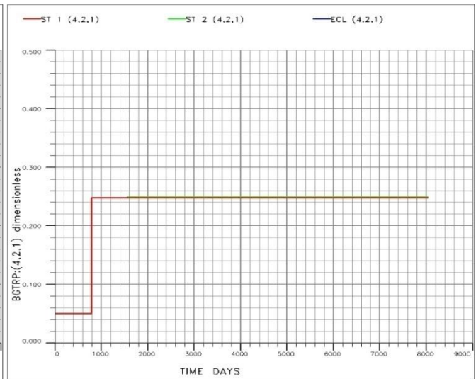
Figure 20: Trapped gas saturation for the grid block (4, 2, 1) VS Time predicted by three methods used.
