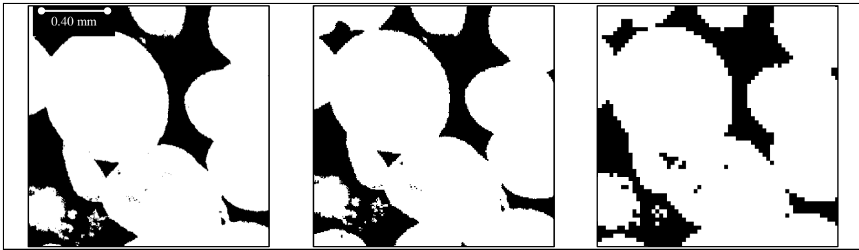
Figure 10. Resolution coarsening effects on Ketton limestone. [Left] original Ketton image of resolution 2.654 \mu\text{m} . [Centre] interpolated Ketton image with an interpolated resolution of 4.42 \mu\text{m} . [Right] interpolated Ketton image with an interpolated resolution of 22.1 \mu\text{m} .
