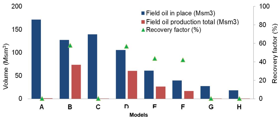
Fig. 9: Production results for all simulation models. The results are shown for field oil in place, field oil production total and recovery factor after 20 years.
