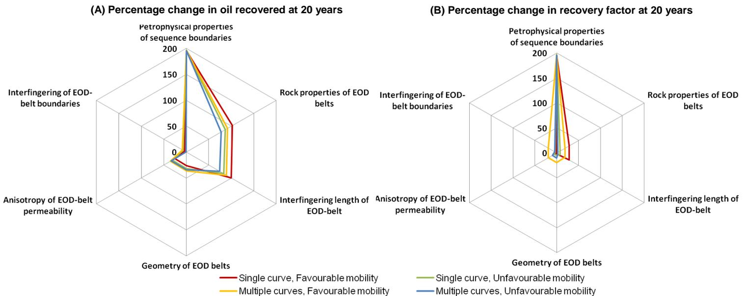
Fig. 13: Impact of six heterogeneities on (A) oil recovered and (B) recovery factor using different relative permeability and capillary pressure models and different fluid mobility ratios. Results are shown for simulations with 4km line drive.
