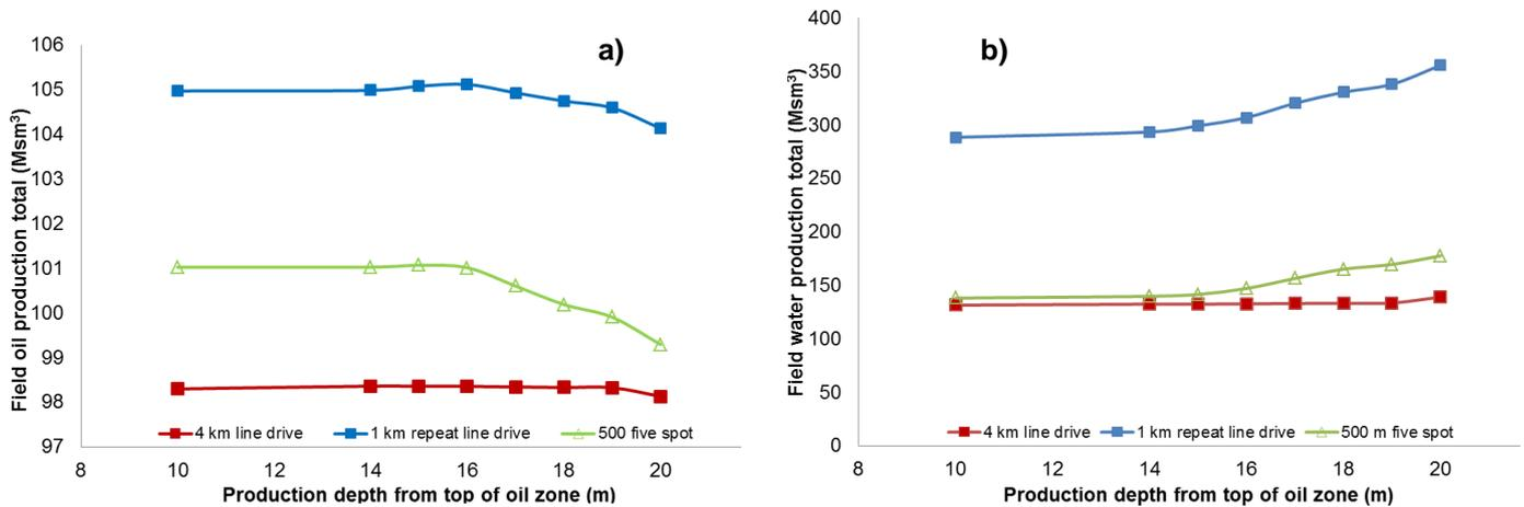
Fig. 7: Sensitivity of production zone to Field oil production total after 20 years (a) and Field water production total after 20 years (b)
