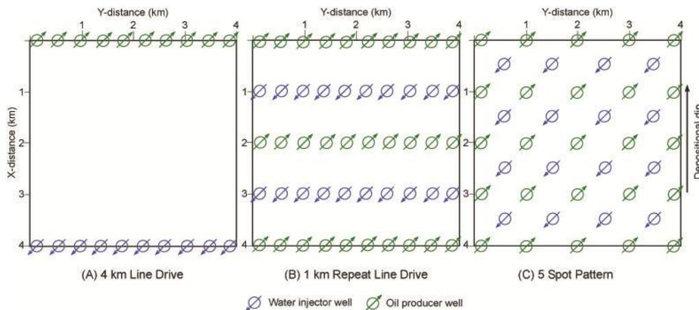
Fig. 4: Plan view showing well spacing and well placement for waterflood development (A) 4km line drive, (B) 1km repeat line drive and (C) 500m five-spot pattern (Fitch et al., 2012)
