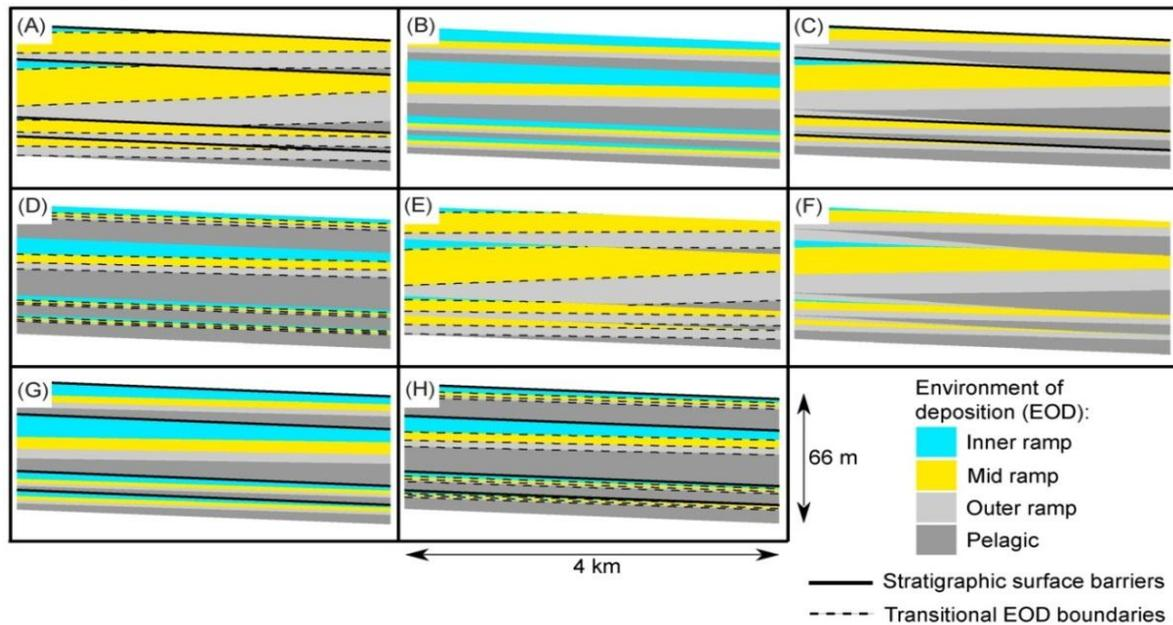
**Fig. 1: 2- D cross-sections showing the combinations of six stratigraphic heterogeneities incorporated into eight models (A–H) (Fitch et al., 2012)**
