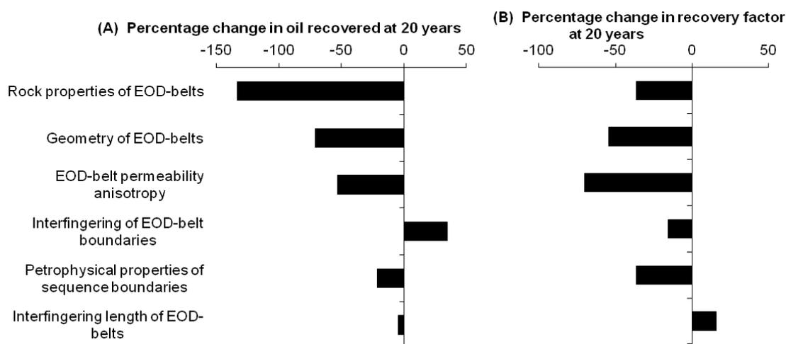
**Fig. 17: Impact of six heterogeneities on oil recovered at 20 years (A), recovery factor at 20 years (B) when the range of permeability anisotropy is increased and the effect of sequence boundary barrier is turned off. Simulations using single imbibition curve set and favourable mobility ratio.**
