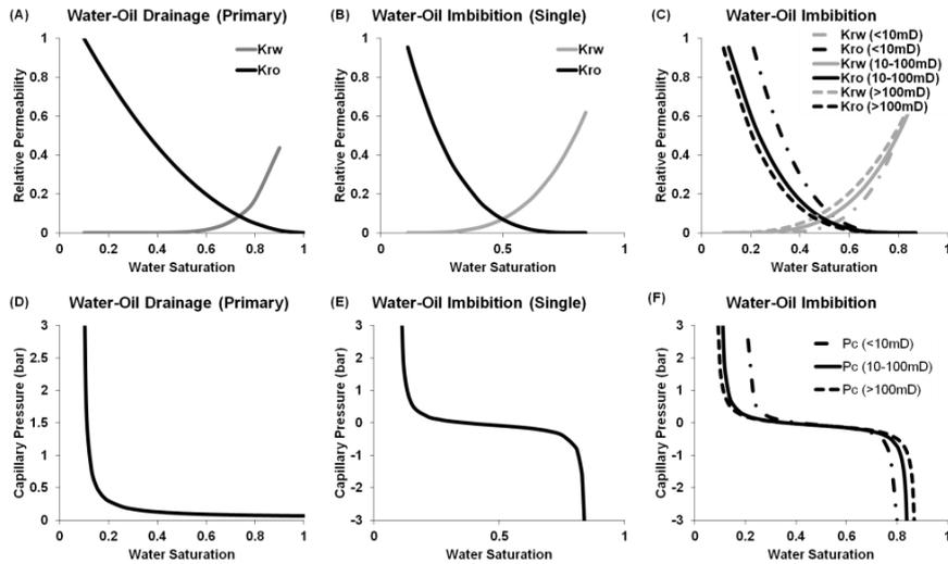
Fig. 3: Relative permeability (A-C) and capillary pressure curves (D-F) used in simulation experiments: primary water-oil drainage curves (A, D); single set of water-oil imbibition curves (B, E); and multiple water-oil imbibition curves (C, F) (Fitch et al., 2012)
