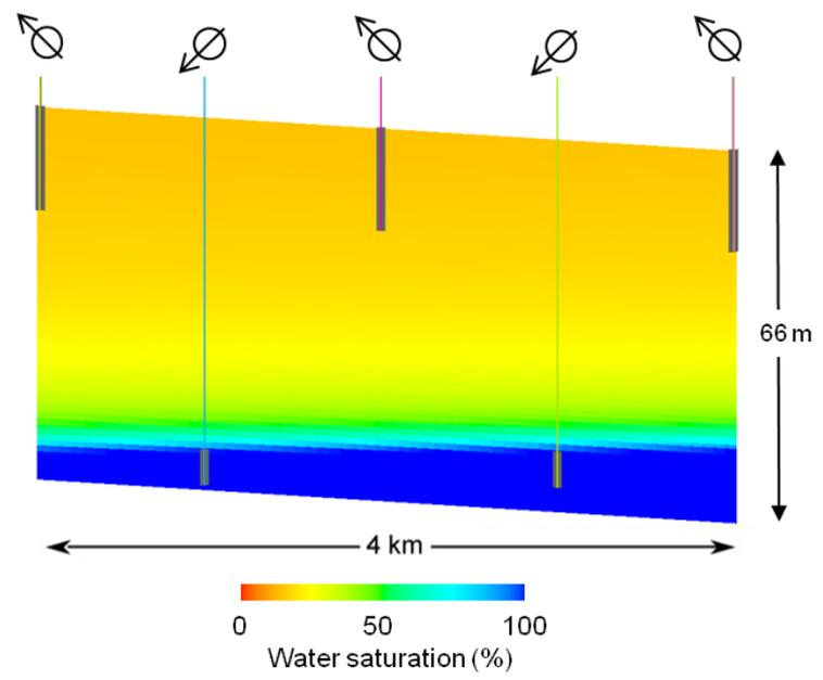
Fig. 6: 2D depositional dip section through the center of a representative simulation model, showing water saturation at the start of simulation. OWC is established. Production perforation is from top of the model and injection perforation is from OWC down to the aquifer.
