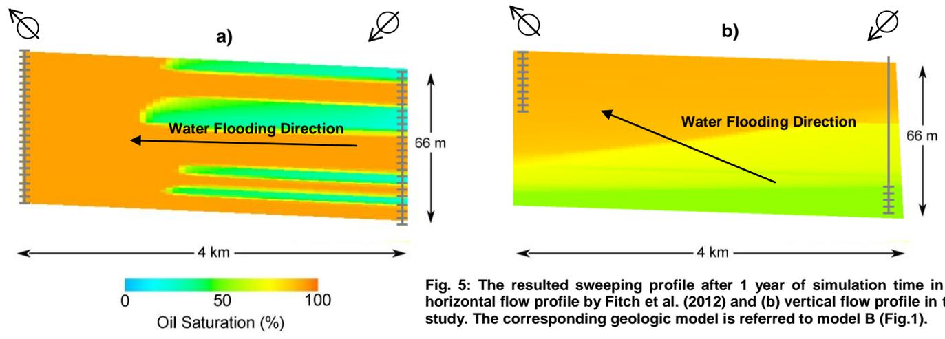
Fig. 5: The resulted sweeping profile after 1 year of simulation time in (a) horizontal flow profile by Fitch et al. (2012) and (b) vertical flow profile in this study. The corresponding geologic model is referred to model B (Fig.1).
