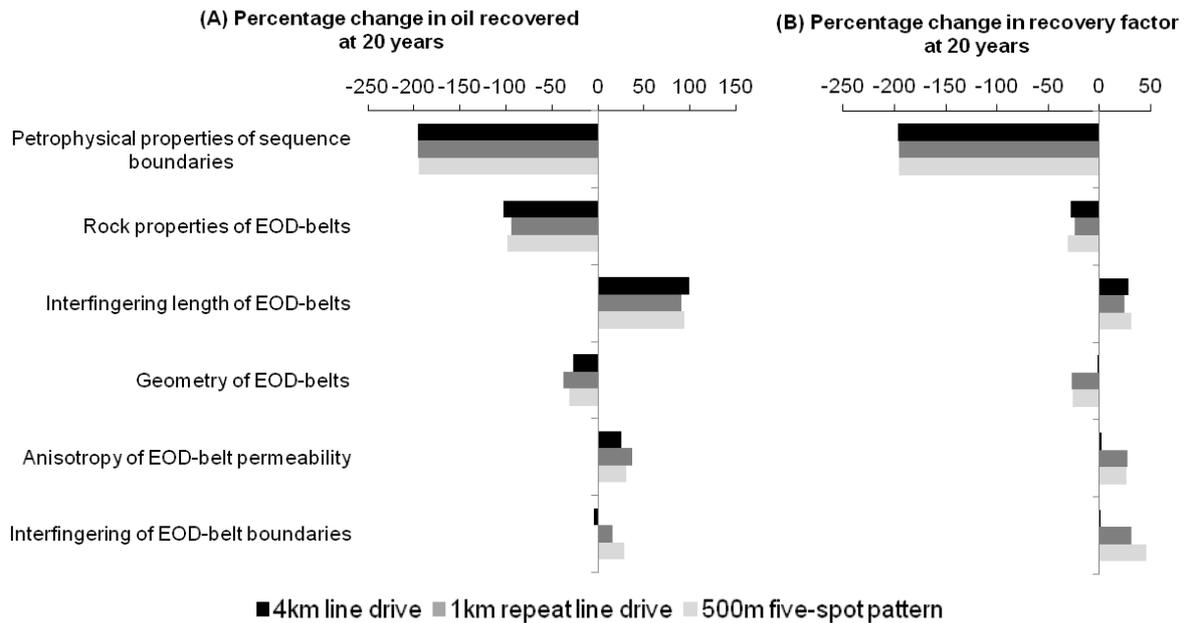
Fig. 14: Impact of well spacing on heterogeneities ranking for (A) oil recovered, (B) recovery factor. Simulations with favourable mobility ratio and single set of imbibition curve.
