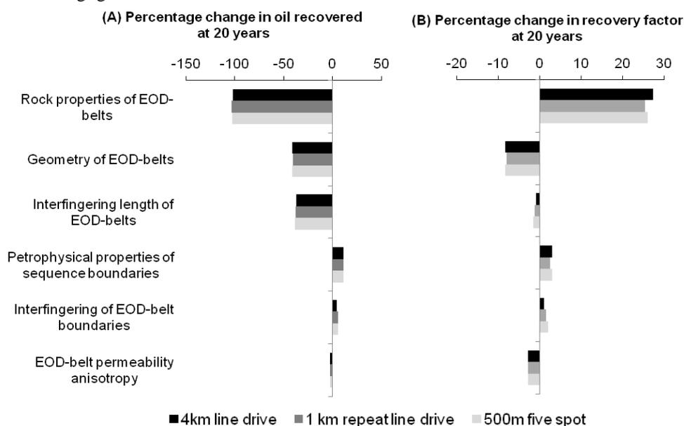
Fig. 16: Impact of six heterogeneities on oil recovered at 20 years (A), recovery factor at 20 years (B) using horizontal water flooding profile (Fitch et al., 2012). Simulation with different well placement using single imbibition curve set and favourable mobility ratio.
