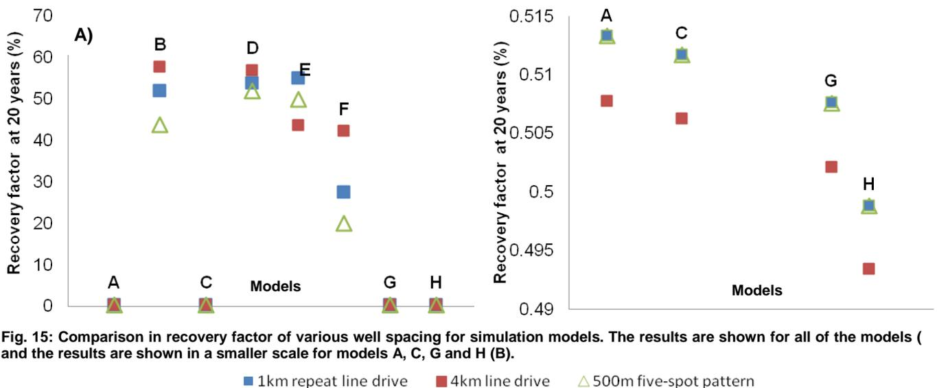
Fig. 15: Comparison in recovery factor of various well spacing for simulation models. The results are shown for all of the models ( Models and the results are shown in a smaller scale for models A, C, G and H (B).
