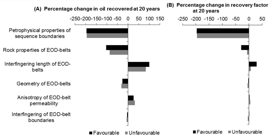
Fig. 12: Impact of six heterogeneities on A) oil recovered at 20 years, B) recovery factor at 20 years. The results are shown for favourable and unfavourable mobility ratio. Simulations with single imbibition curve set and 4km line drive.
