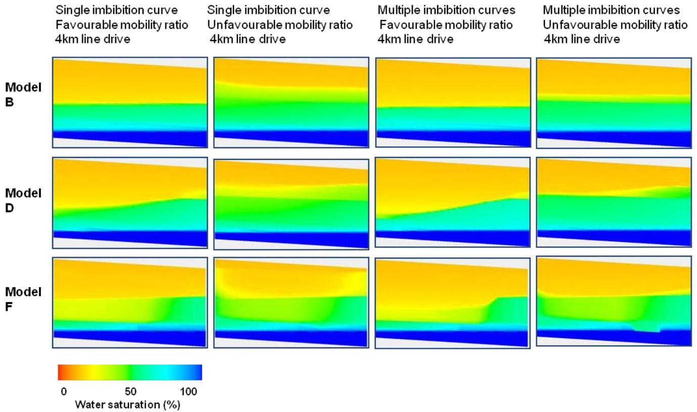
**Fig. B-1: 2-D cross section of models B, D and F without sequence boundary barrier showing water saturation after 1 year of simulation.**
