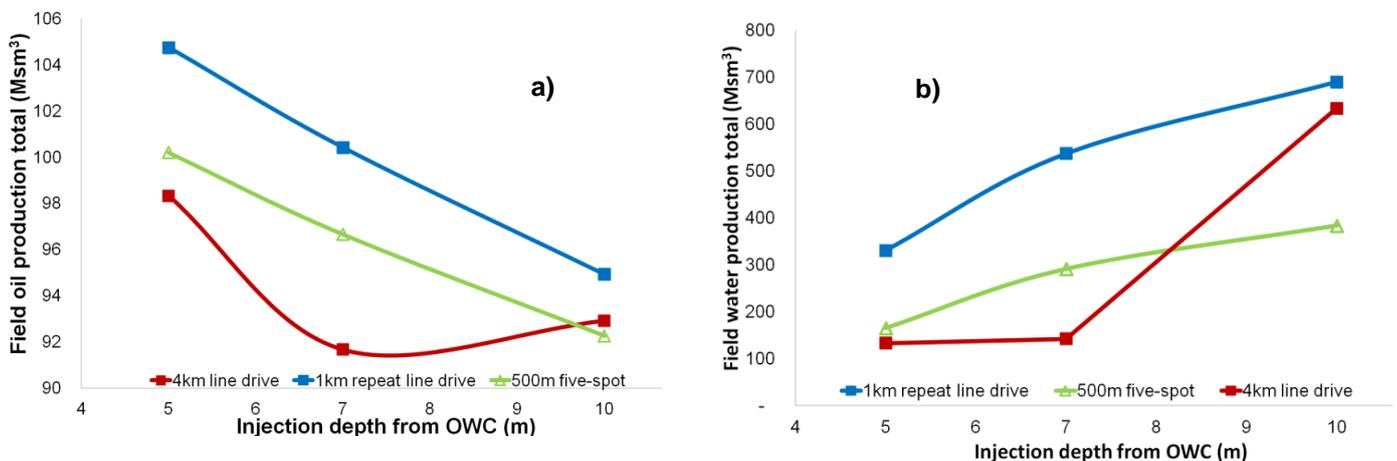
Fig. 8: Sensitivity of injection zone to Field oil production total after 20 years (a) and Field water production total after 20 years (b). All of the production perforations are 16-meter thick.
