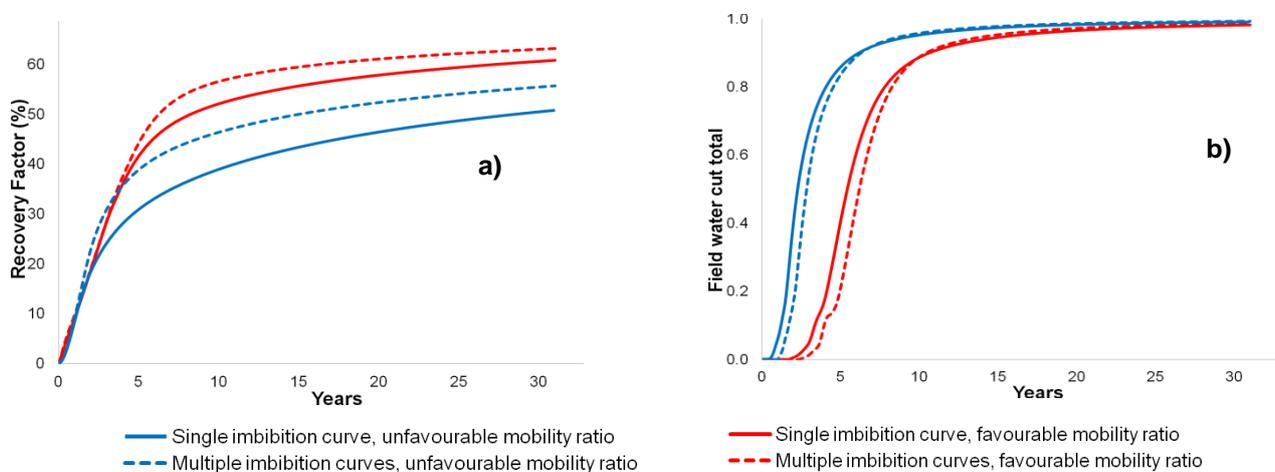
**Fig. 11: Recovery factor (a) and field water cut total (b) for representative model B. The results are shown for single imbibition curve set (continuous lines) and multiple imbibition curve sets (dashed lines). The red lines represent favourable mobility ratio and blue lines represent unfavourable mobility ratio. Simulations with 4km line drive.**
