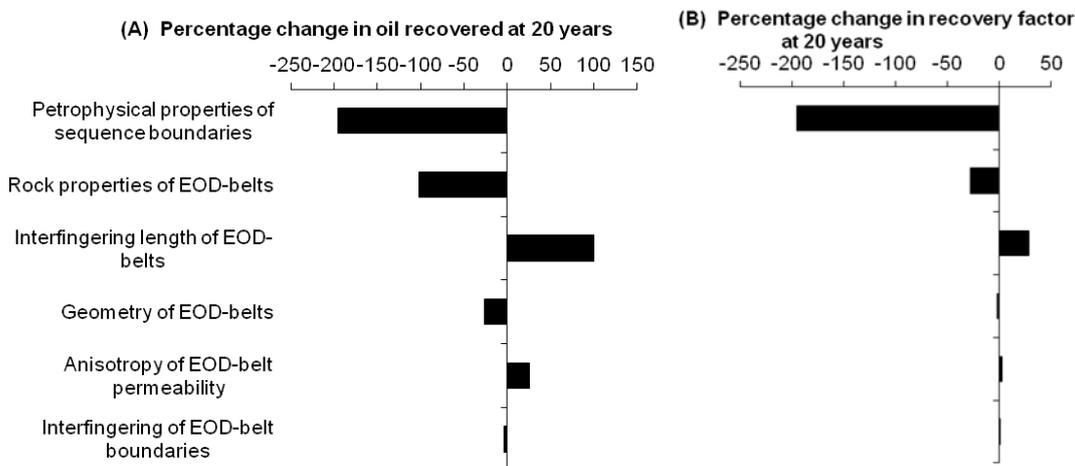
Fig. 10: Impact of six heterogeneities on A) oil recovered at 20 years, B) recovery factor at 20 years. Simulations with single imbibition curve set, favourable mobility ratio and 4km line drive.
