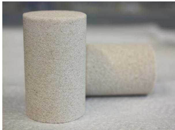
Fig. D1 – Example of Gildehaus sandstone core plug.
