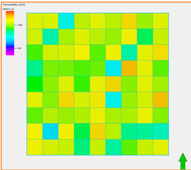
Figure D.15: Effective permeability in Y direction with the No Flow numerical method (in mD)
