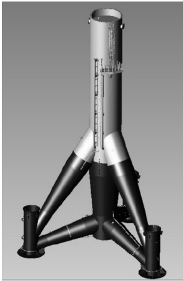
Figure 2: Tripod support structure ( www.weserwind.de )
