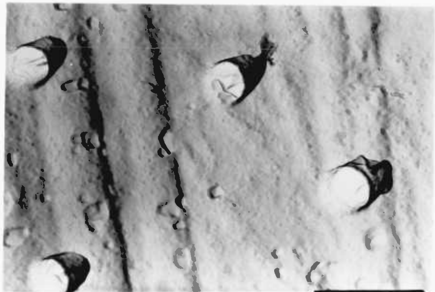
Figure 5.3 k Electron micrograph of 5 MeV alpha tracks in cellulose nitrate (laboratory made) at 45° incidence, etched in 2.5 N sodium hydroxide at 18°C for 26 hours (25 K x 2).
