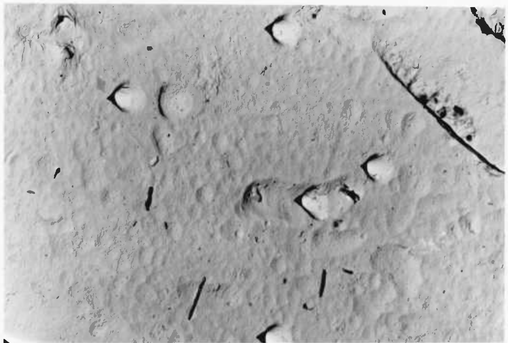
Figure 6.49 Electron micrograph of 1.1 MeV underetched proton tracks in CA80-15 (Kodak-Pathe, France) at 60^\circ incidence, pre-swollen in 65% zinc chloride solution for 2 hours, then etched in 2.5 N sodium hydroxide at 18^\circ\text{C} , for 4 hours (25 K x 3).
