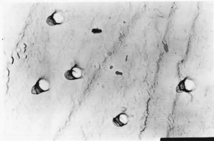
Figure 5.3 g Electron micrograph of 4 MeV alpha tracks in cellulose nitrate (Nixon-Baldwin, U.S.A.) at 45^\circ incidence, etched in 2.5 N sodium hydroxide at 18^\circ\text{C} for 26 hours (25 K x 2).
