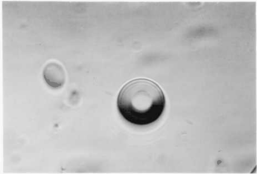
Figure 5.16 Photomicrograph of fission tracks in soda lime glass at 90^\circ and 70^\circ incidence.
