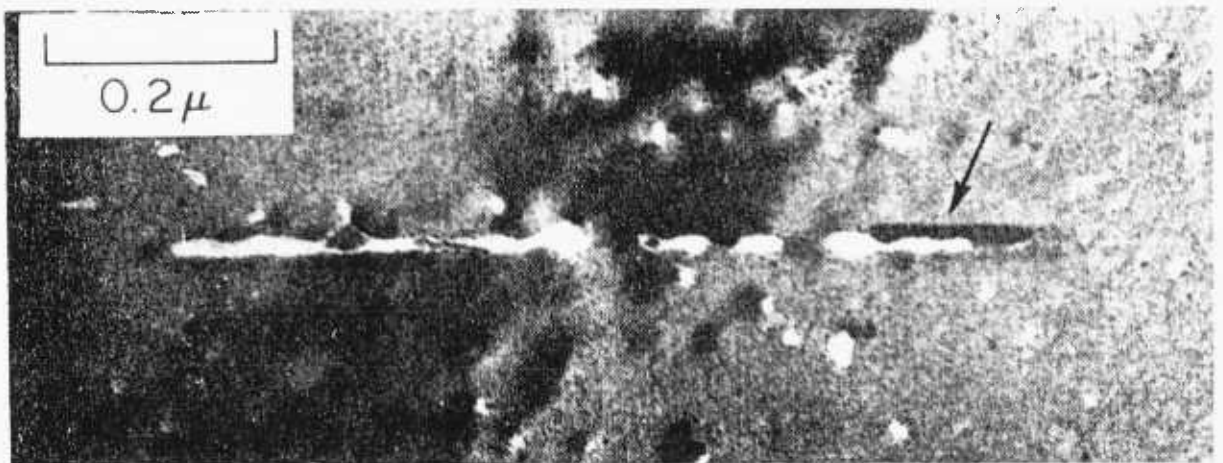
Figure 4.6 Electron micrograph of a thin crystal of lead iodide showing tracks which have 'spikes' at points where the width increases by a factor of two or more. Note that the arrowed track is thinner than those produced by the fission fragments, and is outside the angle of collimation.
