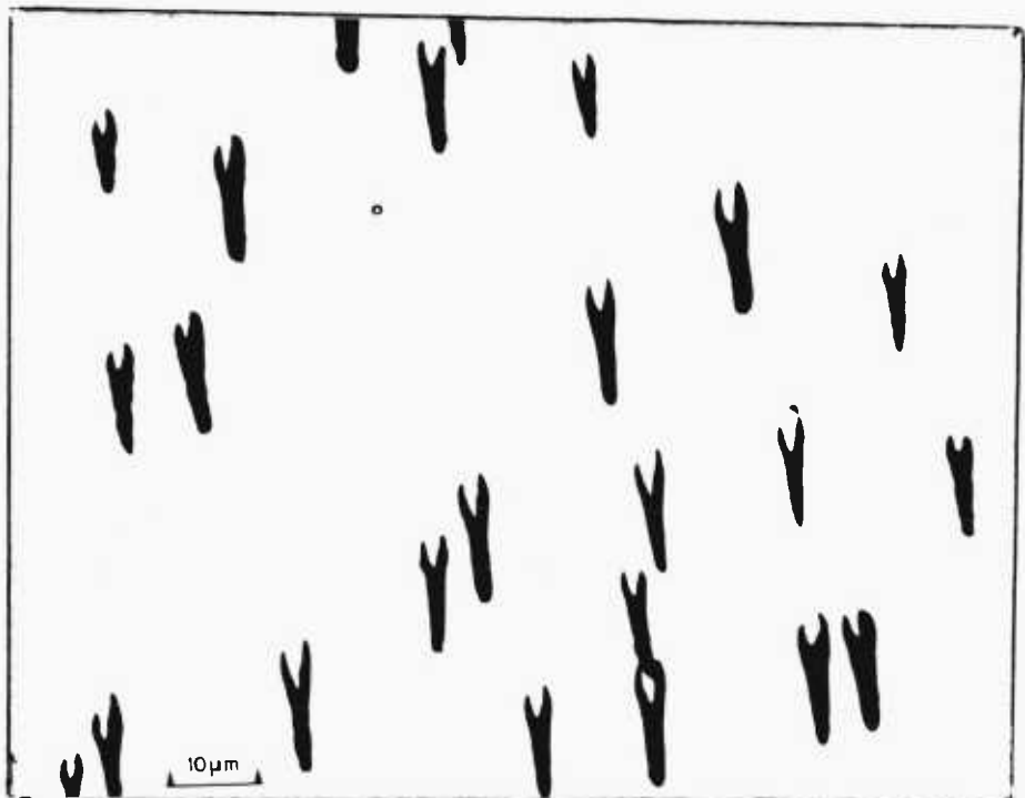
Figure 6.73 Photomicrograph of 4.0 MeV alpha tracks in CA80-15 (Kodak-Pathe, France) at 30^\circ incidence, pre-swollen in 65% zinc chloride solution for 2 hours at 18^\circ\text{C} , then etched in 2.5 N sodium hydroxide at 18^\circ\text{C} for 20 hours.
