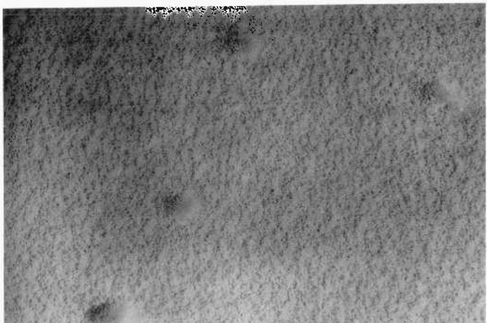
Figure 6.22 Electron micrograph of cellulose nitrate detector, CA80-15 (Kodak-Pathe, France) unirradiated, etched with 5 N sodium hydroxide at 50°C, for 1 hour (25 K x 3).
