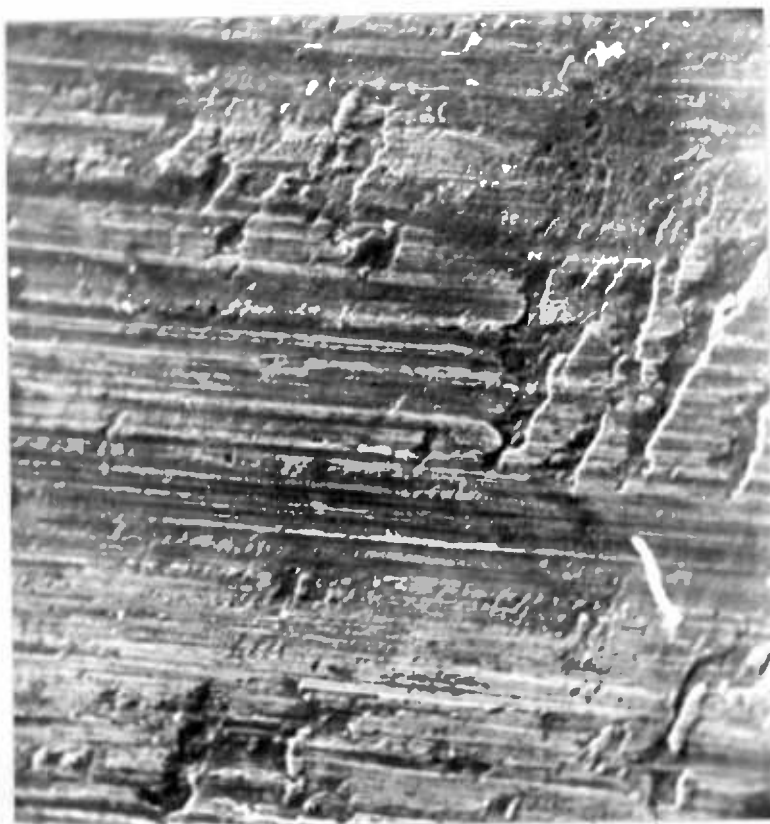
S.E.M. view showing surface flaws left by broaching.
