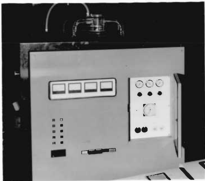
PLATE 4.1B BOC 2kW CW CO 2 laser with power supply and transformer
