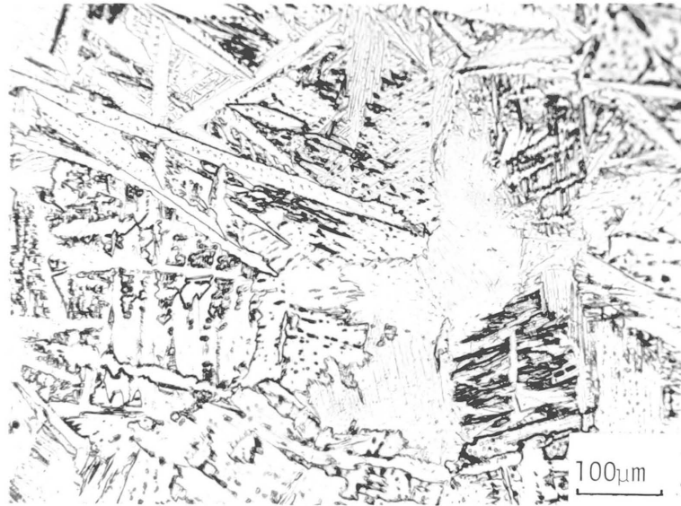
PLATE 7.4 Composite showing structural variation for butt welded 2mm thick CP-titanium (DTD 5063) with CW CO 2 laser welding speed. 11mm/sec, laser power 1110 watts
