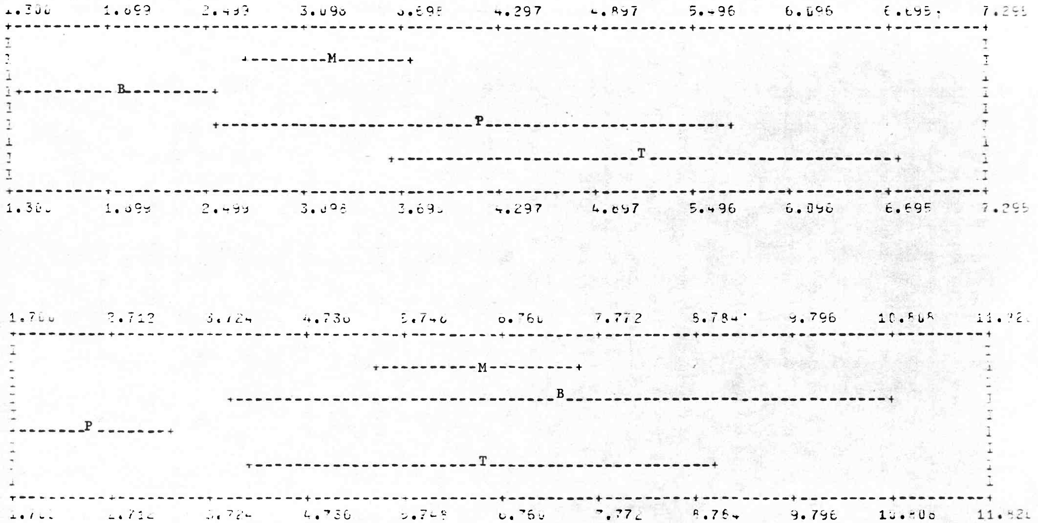
Figure 57: Plot of mean and standard error range of variables determined in random core samples; top Cu s (ppm, scaling factor 10); bottom Fe s (% , scaling factor 10)
