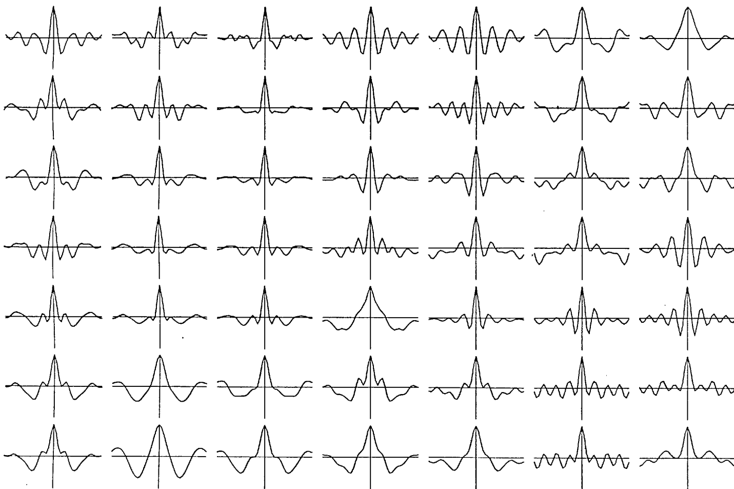
Figure 2.16b The normalized auto-correlation function (ACF) of the second vibration at the measurement sites.
