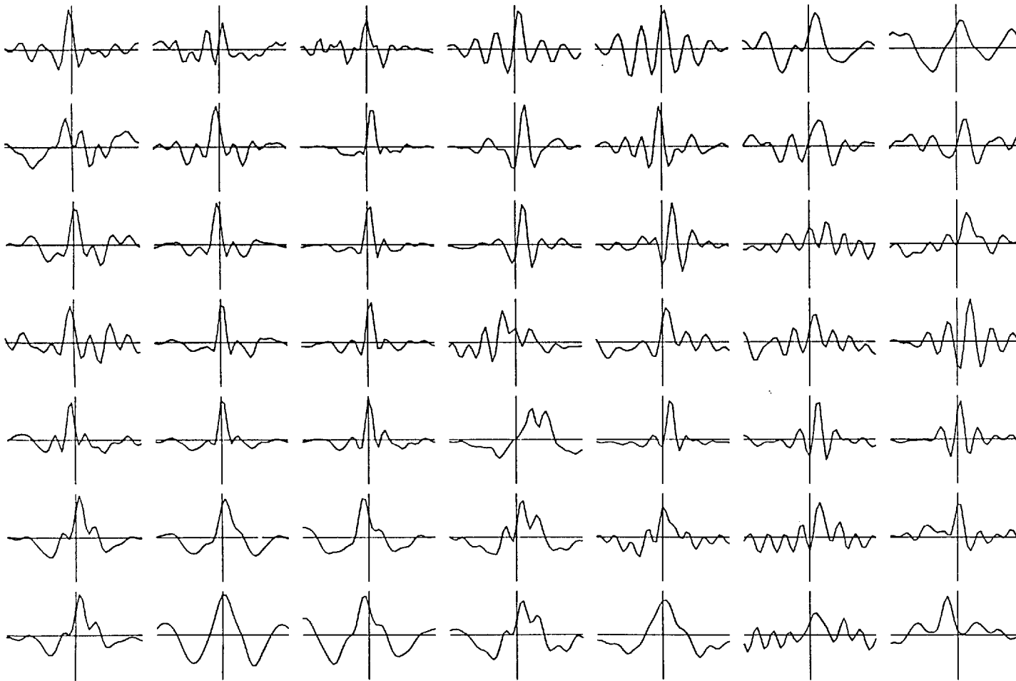
Figure 2.17b The normalized cross-correlation function (CCF) of the averaged measurement between the two experiments. (Second Vibration)
