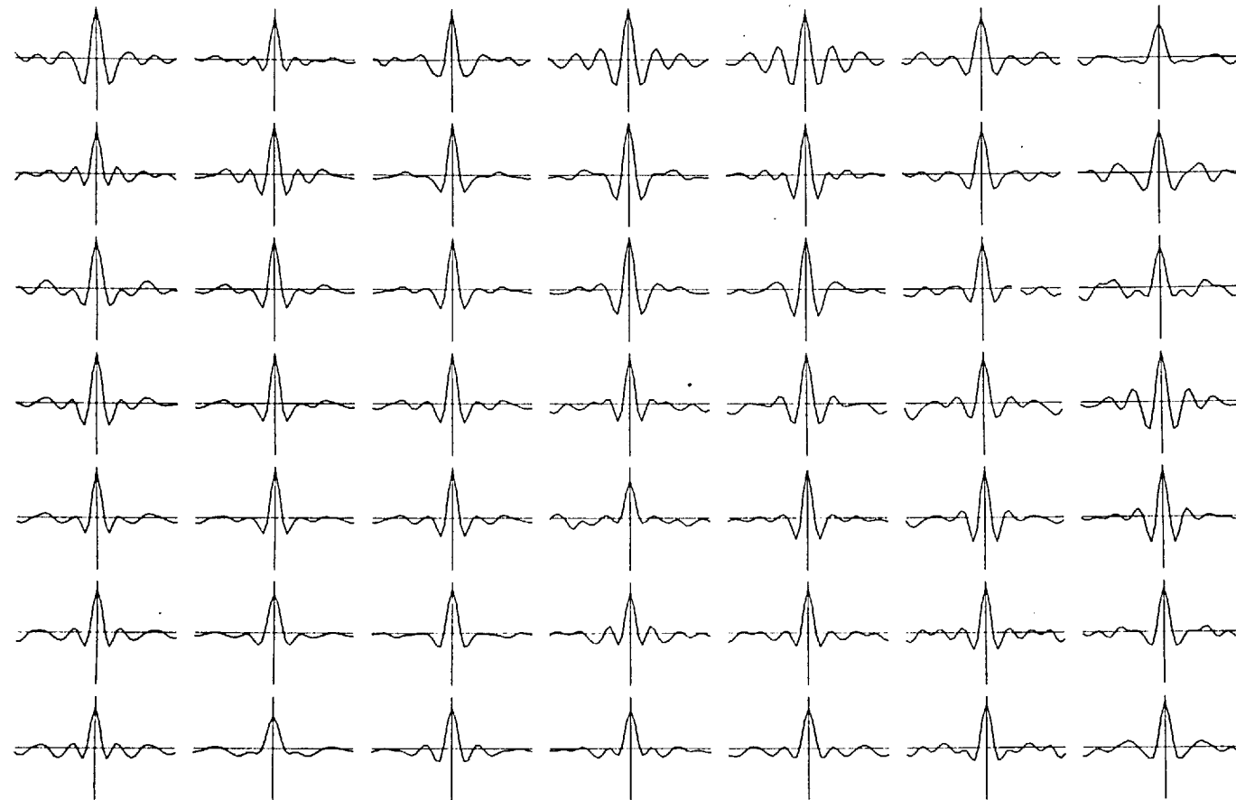
Figure 3.15 The normalized CCF between the observations and signals synthesised from the amplitude spectrum of a reference location (3,4). (compare with figures 1.16 & 3.16)
