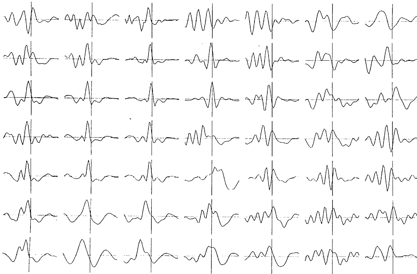
Figure 3.16 The normalized CCF between the observations and signals synthesised from the phase spectrum of a reference location (3,4). (Compare with figures 1.16 & 3.15).
