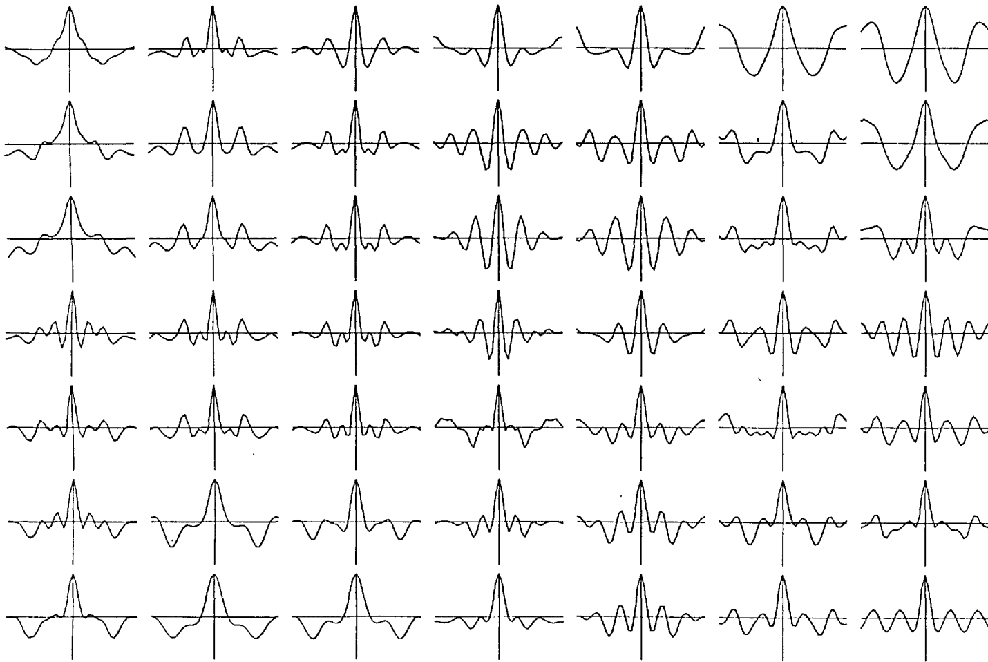
Figure 2.16a The normalized auto-correlation function (ACF) of the first vibration at the measurement sites. (Ordinate normalized to \pm 1 , abscissa shows \pm 20 point shift.)
