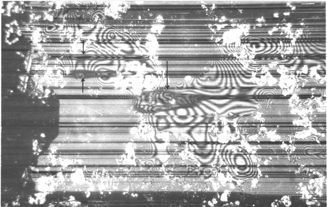
Fig. 6.4. Another interferogram of pumping, note the fringe pattern due to multiple beam interference, x 180.
