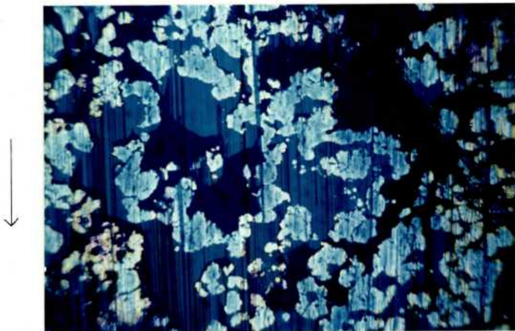
Fig. 5.8. Interferogram of load carrying zone, showing progressive increase of hydrodynamic film thickness as speed increased, x 180, (continued on next page).
