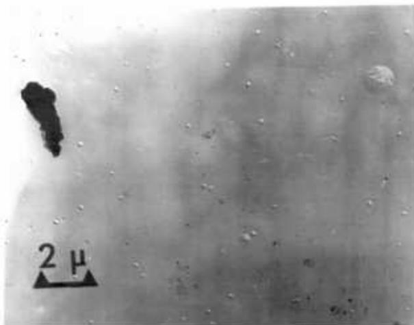
a) Pt/C replica showing  $2 \times 10^7$  pits  $\text{cm}^{-2}$
