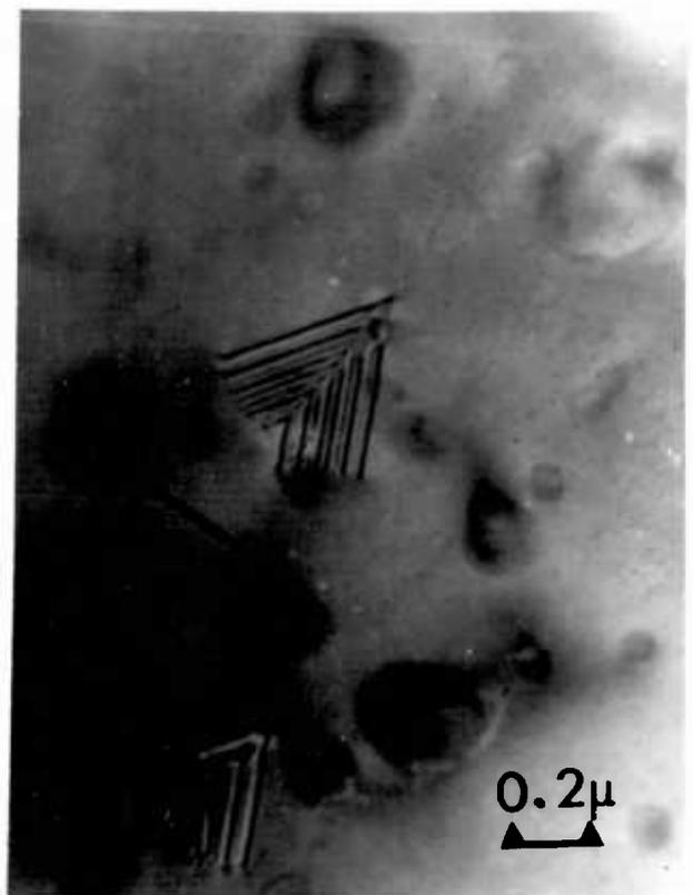
d) as c) showing examples of intersecting faults.
