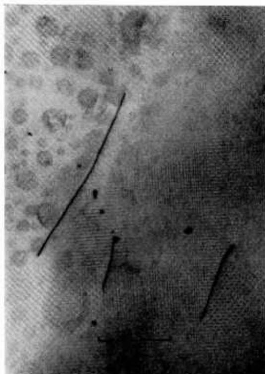
Figure 2 Transmission electron micrograph of dislocation loops.  $220$  type reflection, bright-field. Bar = 1  $\mu\text{m}$ .
