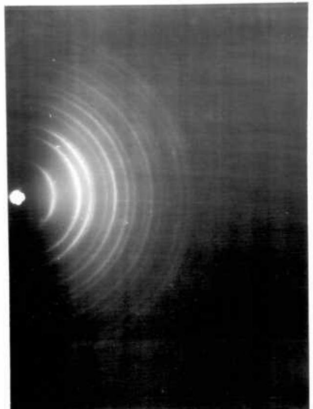
d) Glancing angle electron diffraction pattern of layer.
