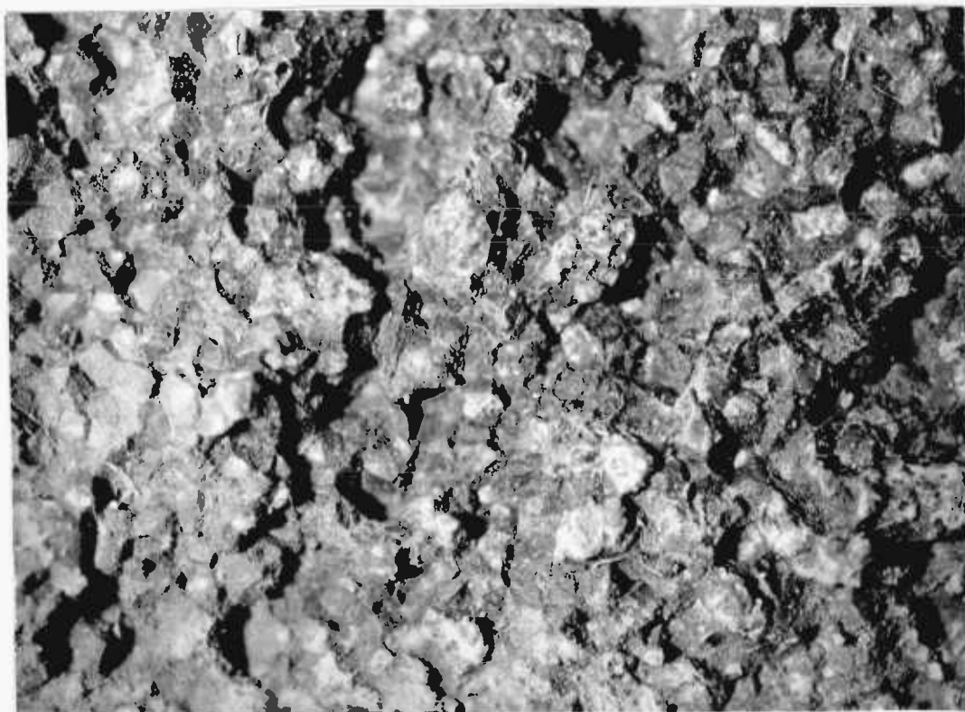
Figure (89): Fracture Surface of the Quenched Steel Creep Cracked at 565°C in air
