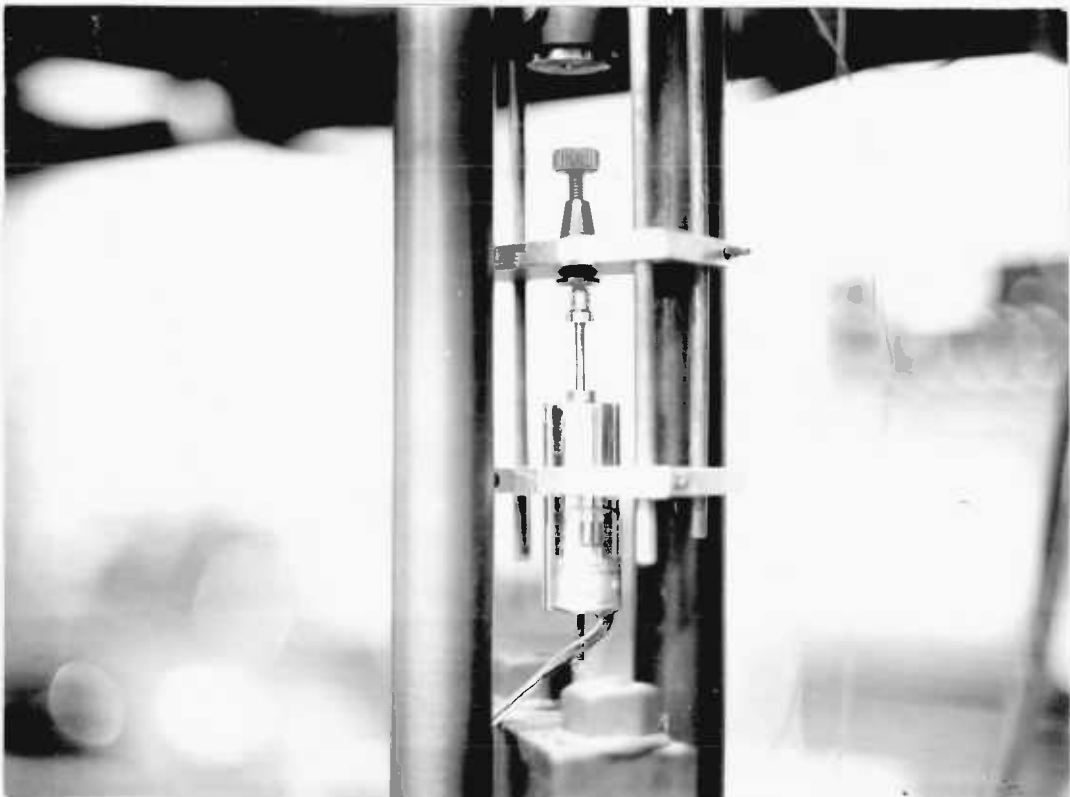
Figure (25): View of the transducer set-up, below the furnace, used to measure the displacement at the loading line of specimens
