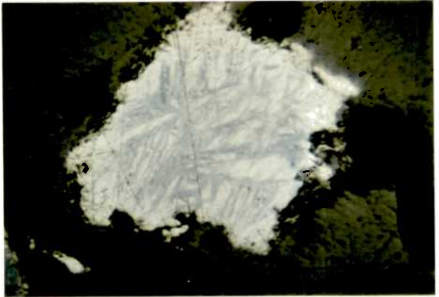
FIGURE C-2.10 : Stromeyerite leach residue (77.58% Cu dissolved), showing the attack at the edges of the particles.
