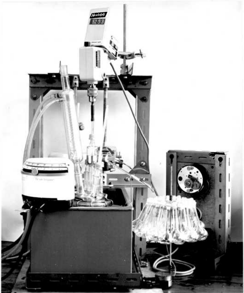
FIGURE 22 : The Leaching Apparatus. The set-up to the right of the oil bath could be used for automatic sampling of the leach solution.
