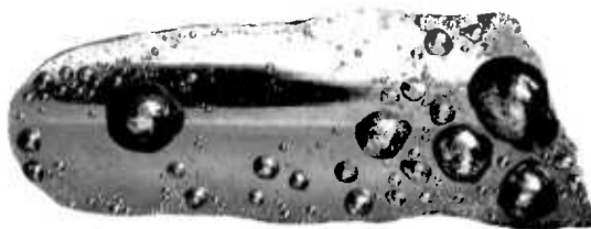
FIGURE 21 : (a) External appearance of synthesised Mixed Sulphide Material, upper and lower surfaces (approx. x2). (b) Cross-sectional view of Mixed Sulphide Material (approx. x5). (c) External appearance of synthetic Stromeyerite, upper and lower surfaces (approx. x2). 'Wire' silver in upper piece, upper left hand corner.
