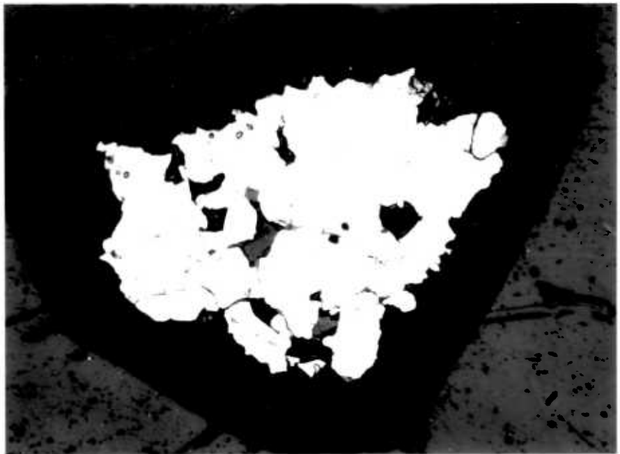
FIGURE C-2.4 : Silver-doped bornite leach residue (84.04 wt.% Cu dissolved), showing the hole left by the removal of the sulphur layer during polishing.
