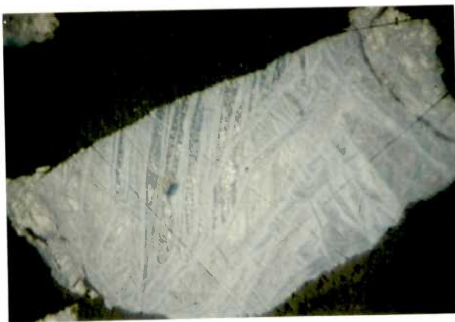
FIGURE C-2.9 : Stromeyerite leach residue (50.06% Cu dissolved), showing the fine intergrowth of the blue phase and a light-coloured phase.
