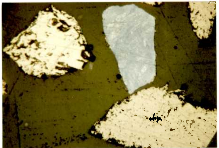
FIGURE C-2.23 : One particle of (from l. to r.) chalcopyrite, stromeyerite, and bornite from a mixture of separate particles of the minerals after leaching in a 0.25M \text{Fe}^{3+} (pH 1) solution at 60°C.
