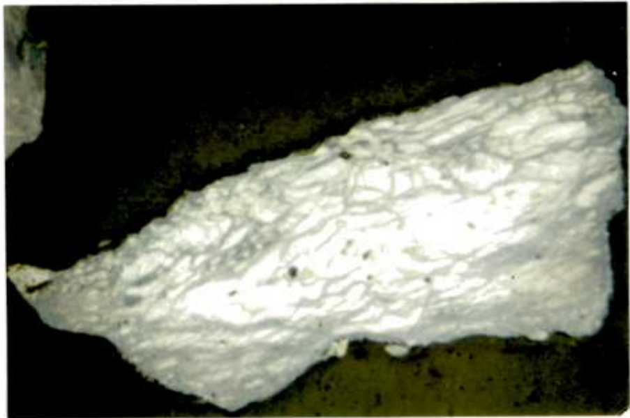
FIGURE C-2.7 : Stromeyerite leach residue (26.15% Cu dissolved), showing the increase in the amount of the blue phase as more Cu dissolved.
