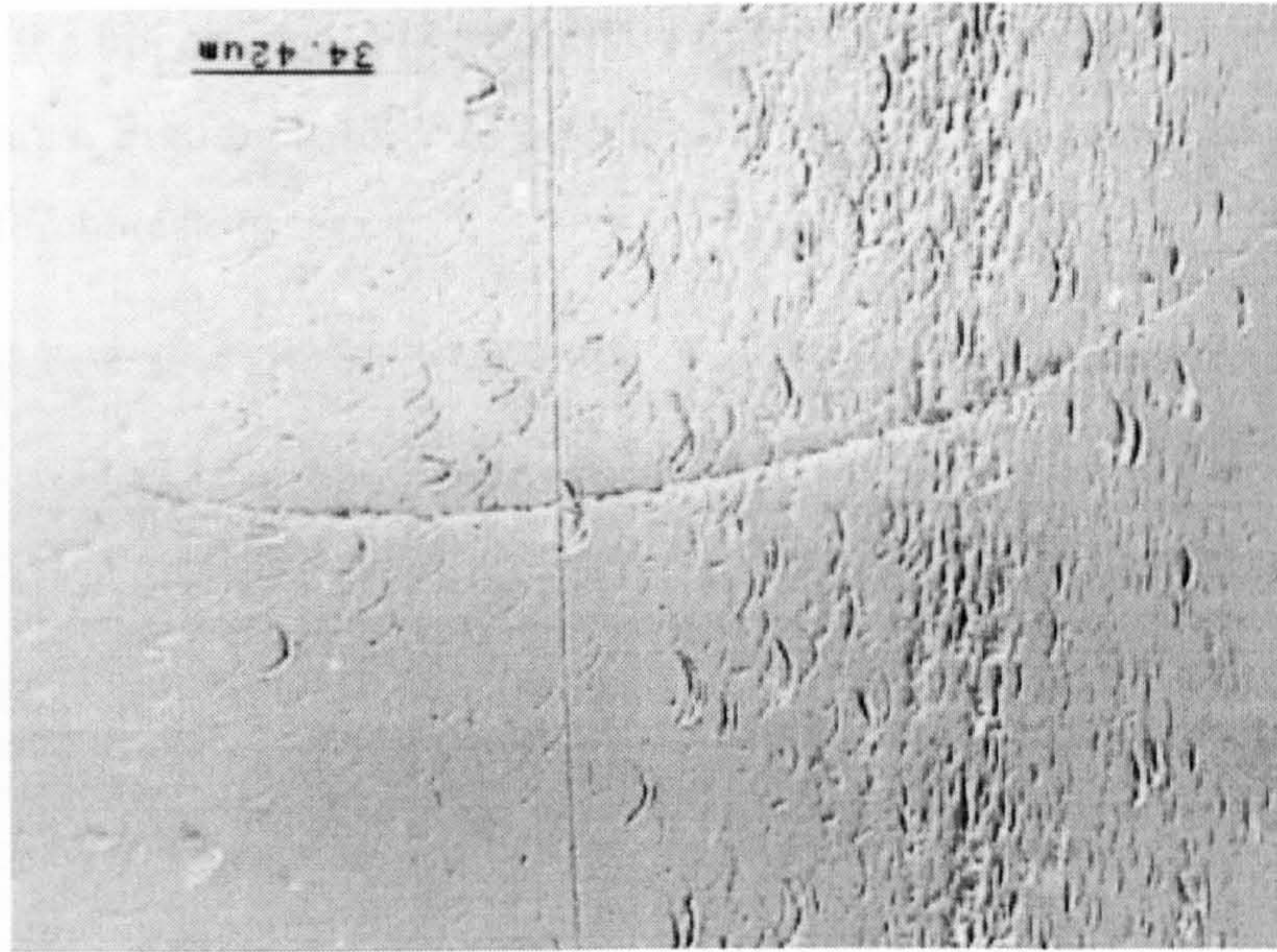
(e) Detailed views of the contact track after deposit removed
