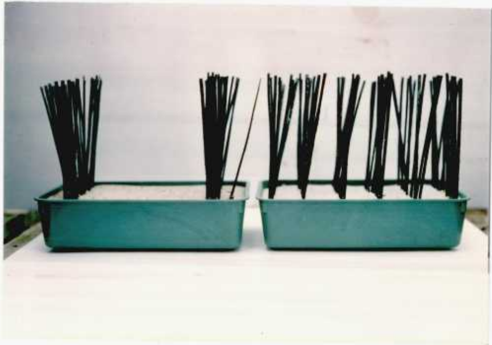
Plate 11. 'Artificial plants' in rows spaced 15cm apart (left) and in rows spaced 5cm apart (right). Sixty-four 'artificial plants' per tray.
