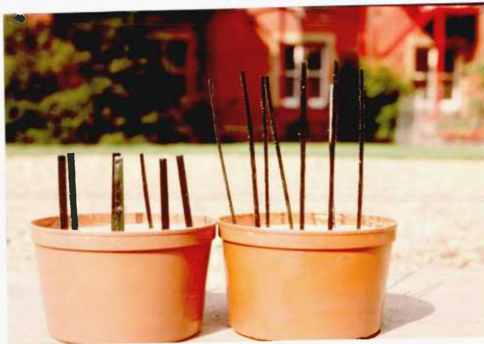
Plate 8. 'Artificial plants' of different heights (left: 6.5cm; right: 13.0cm) but the same area ( 4.23\text{cm}^2 ).
