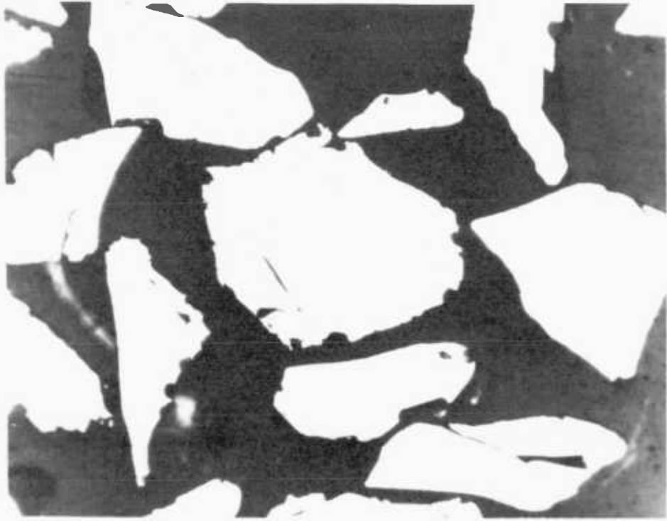
FIG. C-2.1 Unleached Sample of the Monosulphide Solid Solution of Nickel and Iron (Mss)
