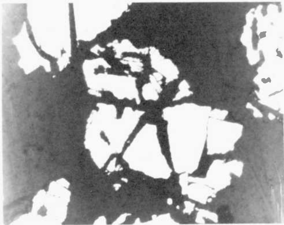
FIG. C - 3.4 Pentlandite Leach Residue from which about 20% Nickel was Dissolved
