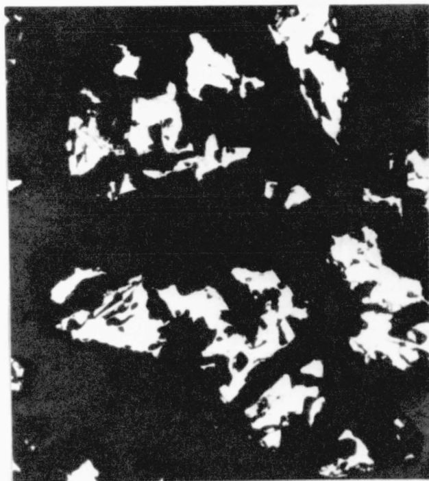
FIG. C - 3.6 Pentlandite Leach Residue from which about 70% Nickel was Dissolved
