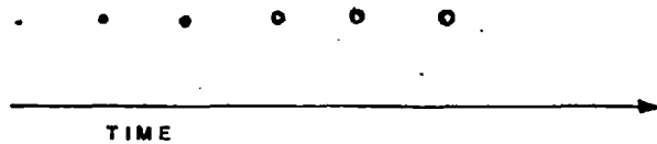
Figure 6.5 The variation in the diameter of char prints from the same beam with the exposure time.
