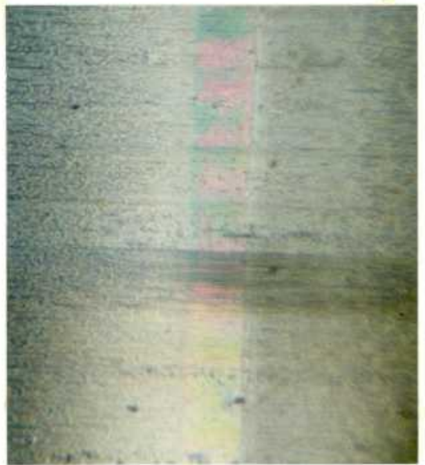
(d) 576 R.P.M. 2nd Green, X_i = .0015 in., h_0 = 15.8 \mu in. 2nd Red, X_i = .0006 in., h_0 = 12.8 \mu in. 2nd Yellow, X_i = .0002 in., h_0 = 11.1 \mu in.
