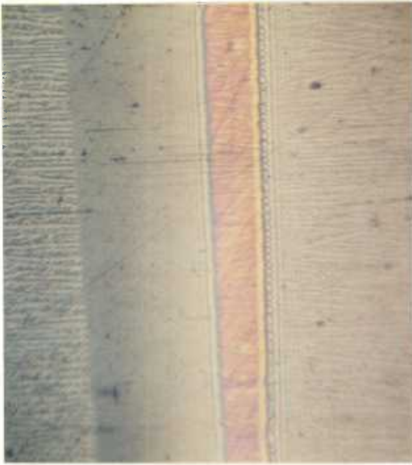
(a) 31 R.P.M. 1st Red, X_i = .027 in. h_0 = 6.3 \mu in.
