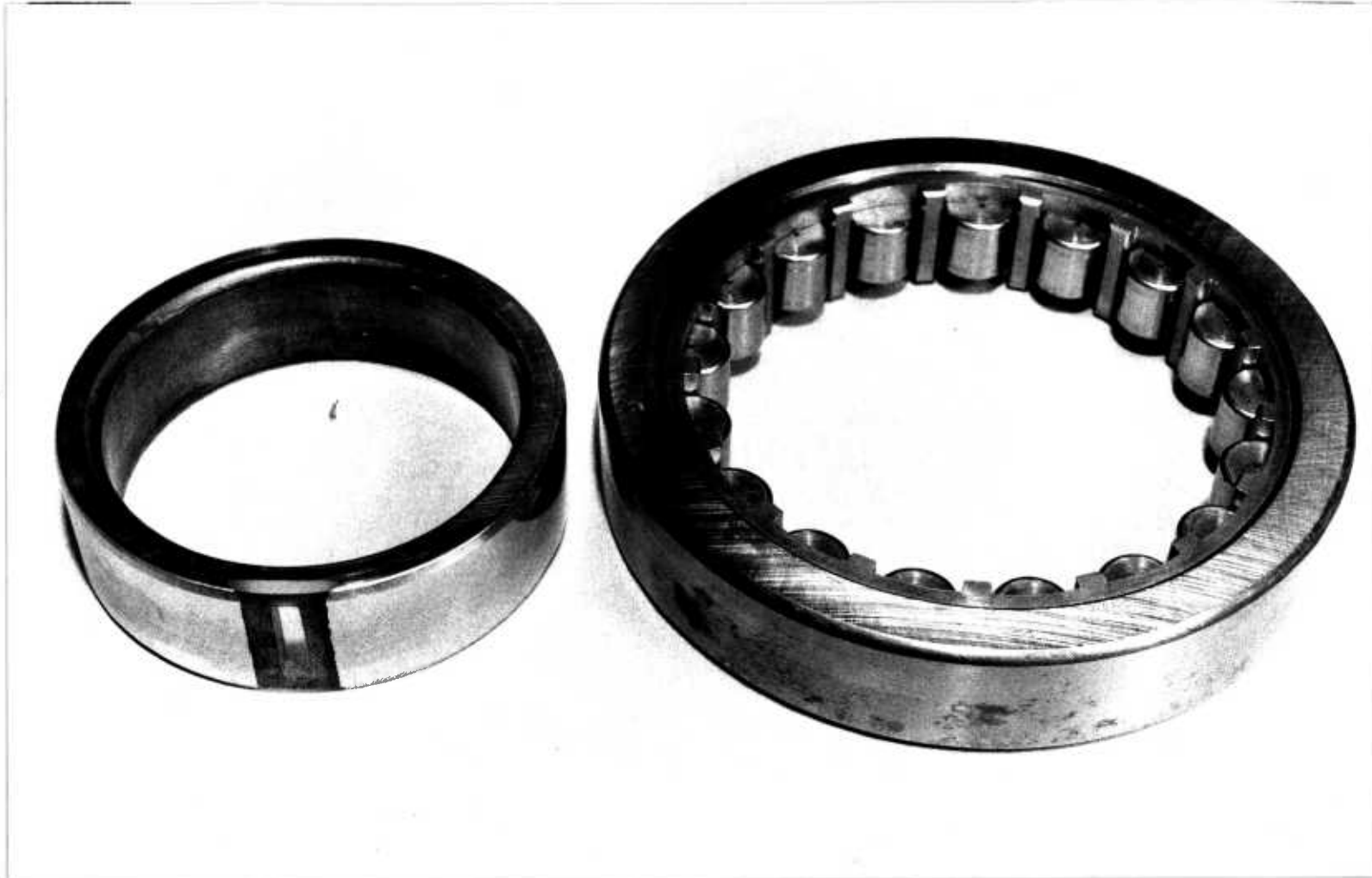
Figure 3.7 Test bearing for optical study of the inner race.
