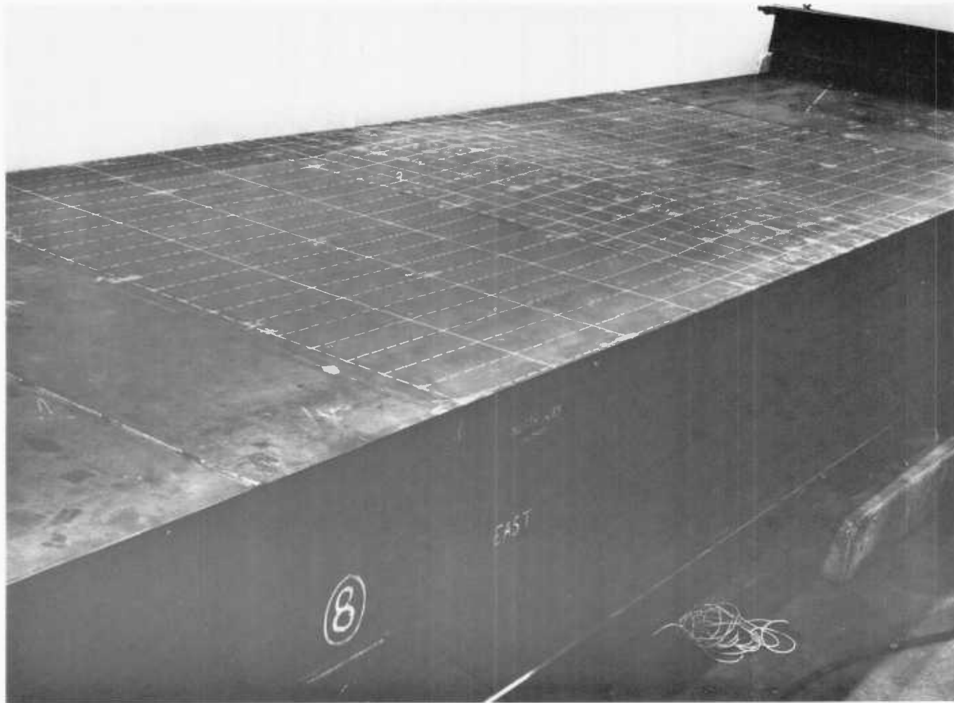
Fig. 2.90a. Model 10 - a view of the model after the collapse test (Test 10C). Stiffener locations are indicated by dashed lines.
