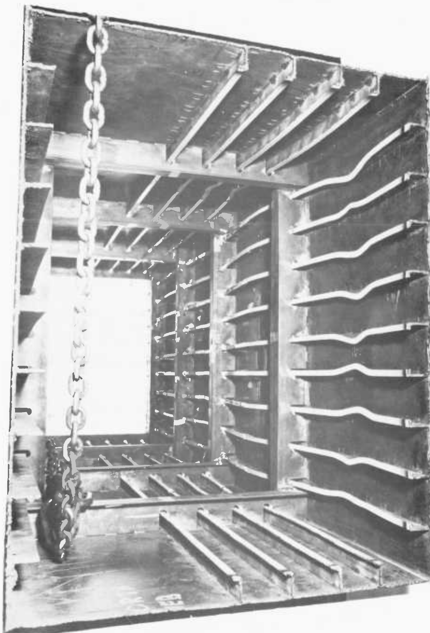
Fig. 2.43b. Model 4 - an interior view of the model (from end A) after failure.
