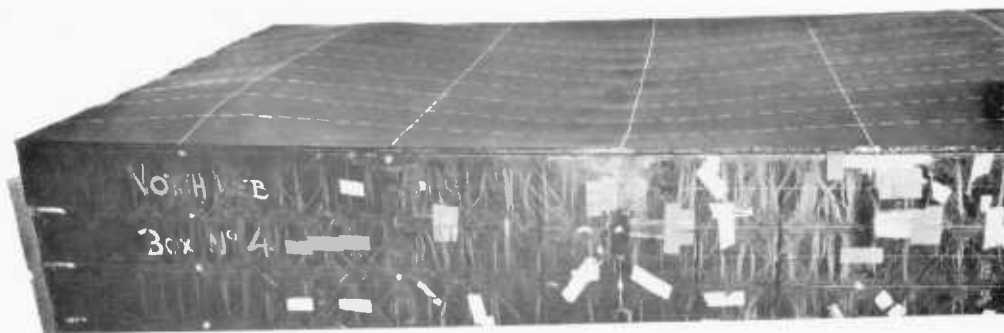
Fig. 2.43a. Model 4 - showing part of the compression flange after the test to failure. Stiffener locations are indicated by dashed lines.
