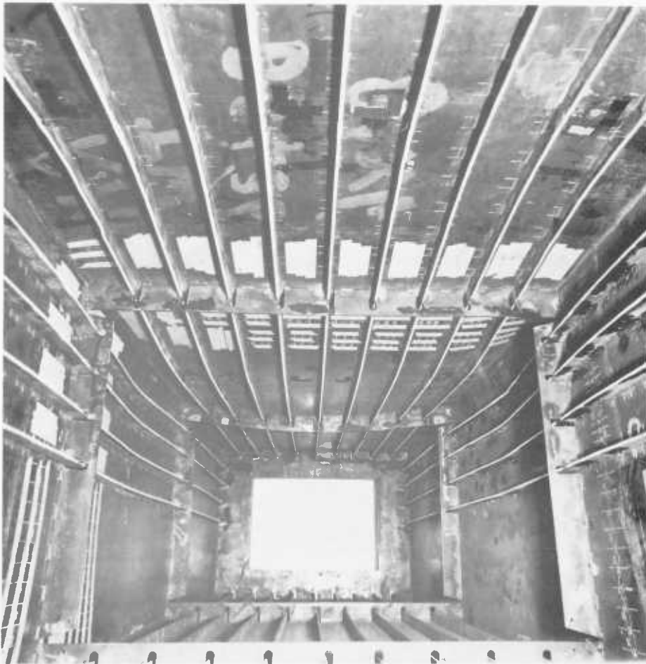
Fig. 2.52b. Model 8 - showing the inside of the model (from end M) after failure. The compression flange is at the top of the picture. Although the deflections in bay I-M were outwards, the longitudinal stiffeners exhibit very little lateral deflections.
