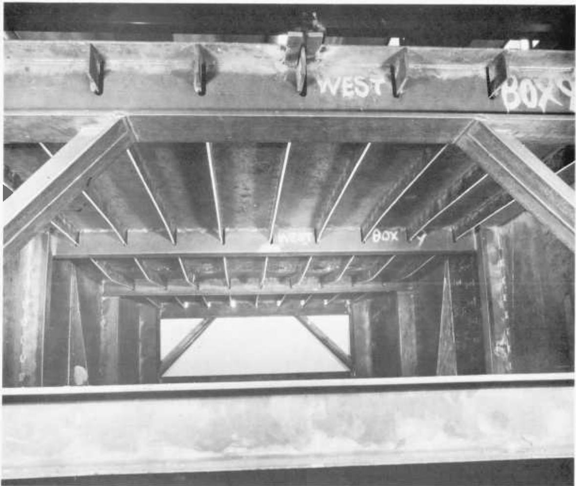
Fig. 2.67c. Model 9 - an inside view of the model (from end A) after collapse.
