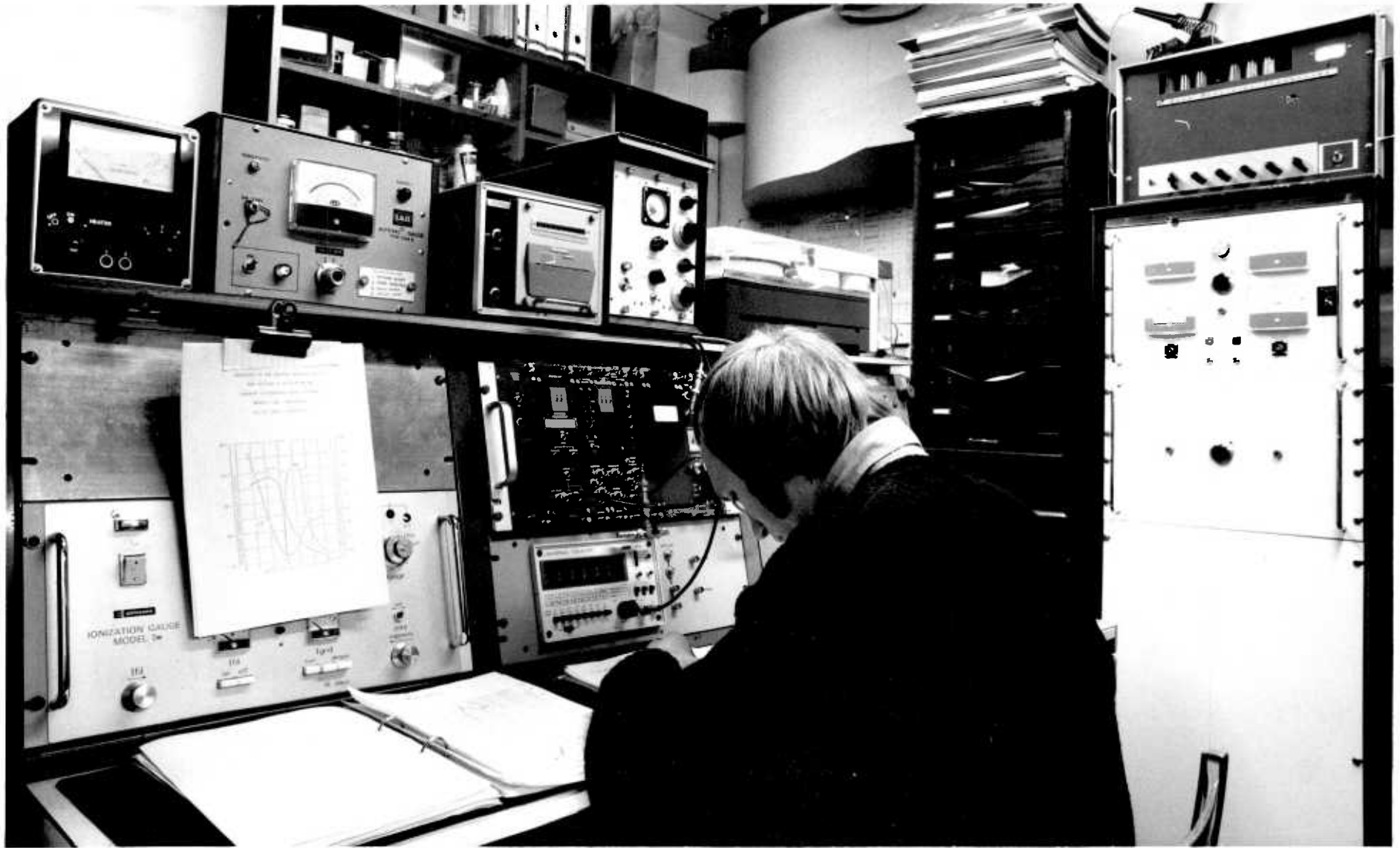
FIG. 84 THE GRATING TEST APPARATUS: CONTROL CONSOLE
