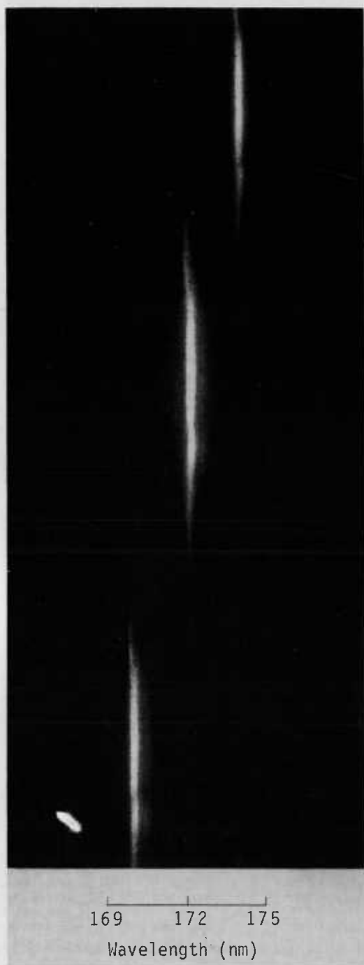
Fig. 2. Output spectra of VUV xenon laser showing frequency narrowing and tuning. The spectrograph plate was moved vertically between recordings and the tuning prism rotated.
