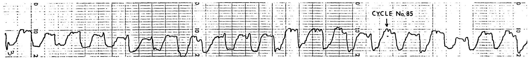
FIGURE 6.11-5b Pseudo-steady state liquid profiles for outlet stream illustrating the effect of small disturbances.
