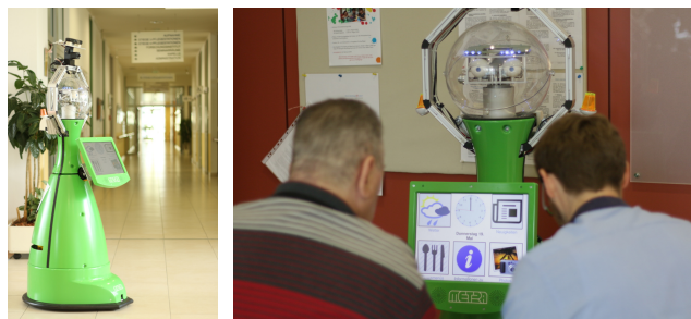
(a) Robotic platform. (b) Subject using the developed info-terminal using touch-screen interaction.
