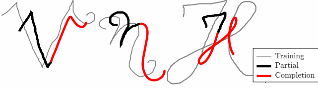
Fig. 3. Phase estimation and pattern completion using DTW and DMPs. Given the partial observation (black), we estimate the current phase, and use it to generate the unseen part (red) of the letter. The goal does not have to be specified and is estimated alongside the other parameters.
