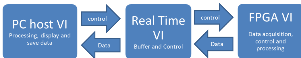
Figure 3-14: Hierarchy of control and data transfer of the three levels of LabVIEW VIs.
