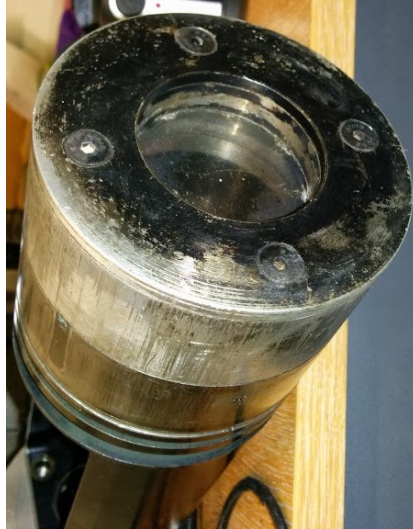
Figure 3-4: Image of the piston showing a cylindrical piston bowl and a quartz window at the bottom of the bowl.
