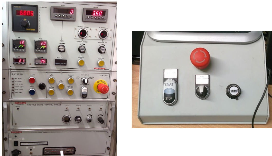
Figure 3-13: Front panel of the Cussons main control unit (left) and the remote control outside the test cell (right).
