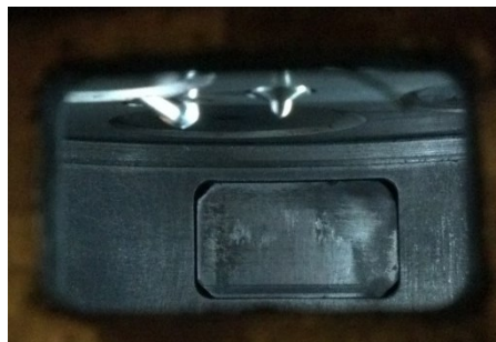
Figure 3-19: Drawing of the windows carrier (combustion chamber annulus) for the Hydra and a view into the combustion chamber through the side window. A metal blank can be seen through the window on the opposite side of the bore.
