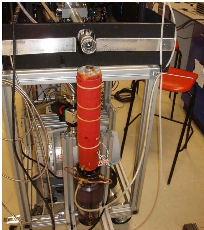
Figure 2-14: Aerosol generator with heater (orange part).
