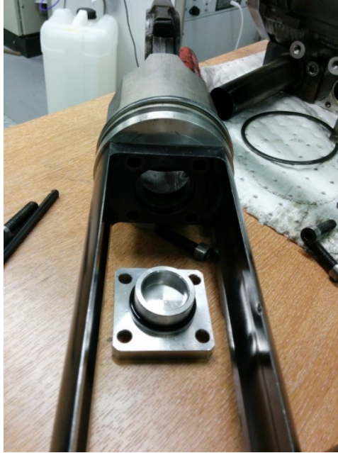
Figure 3-8: New sealing plate with O-ring connecting the Bowditch extended optical piston to the bottom piston.
