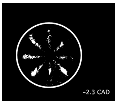
Figure 7-25: Visualisation of diesel spray injected at -5CAD after the first injection at -10CAD, -15 CAD and -20CAD.
