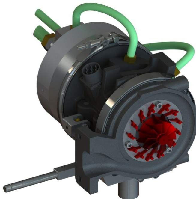
Figure 4.1 - 3D drawing of the turbine tested. The volute has been cut to show the vanes and the rotor, which are coloured in red
