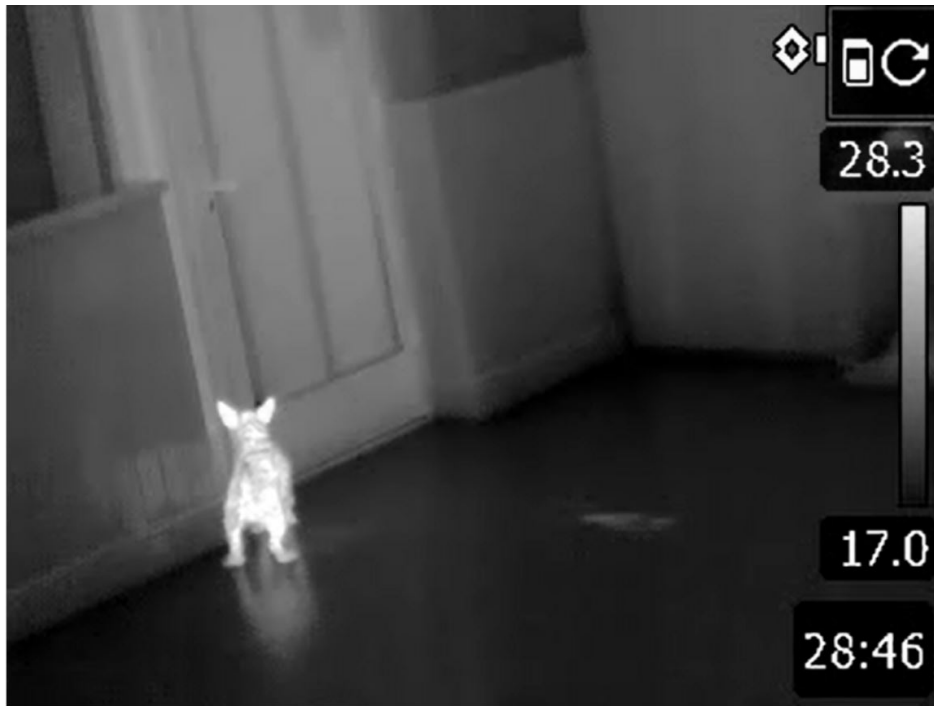
Figure 2: Example of the view of the thermographic camera (settings at gray-scale for subsequent analysis; brighter colors correspond to higher temperatures as indicated on the bar on the right)
